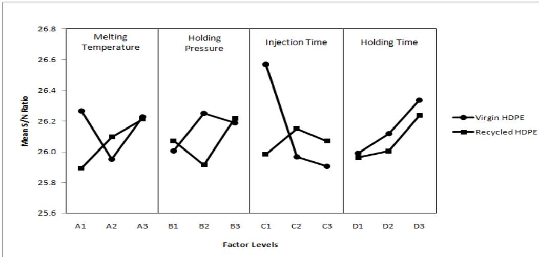
Figure 3: Main effects of tensile strength for virgin and recycled HDPE.
