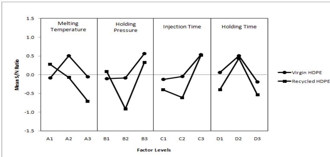
Figure 4: Main effects of compressive strength for virgin and recycled HDPE.
