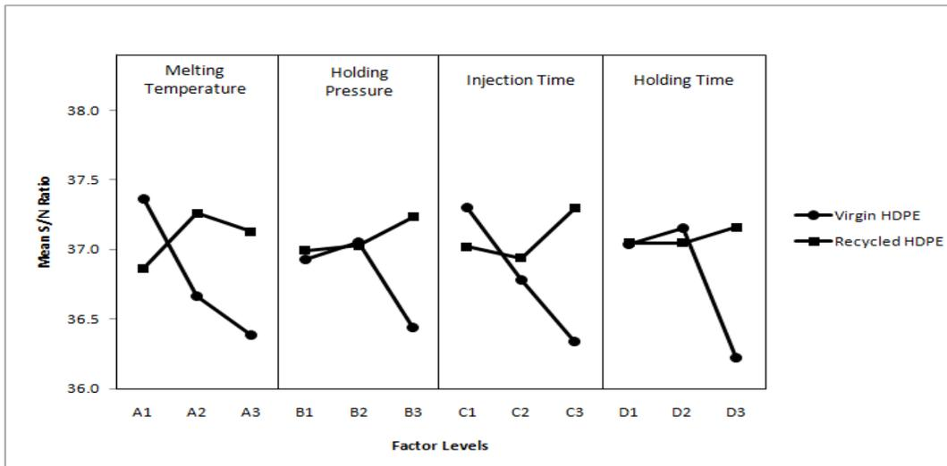
Figure 5: Main effects of flexural strength for virgin and recycled HDPE
