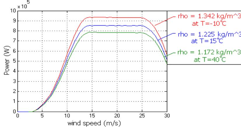
Figure 25 Effect of air density-temperature on the generated power
