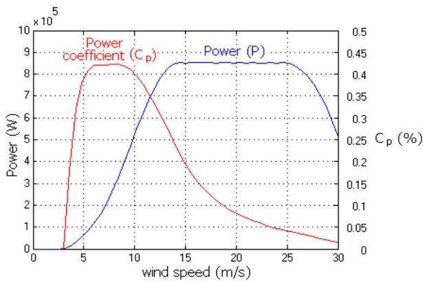
Figure 26 Generated power as a function of the power coefficient
