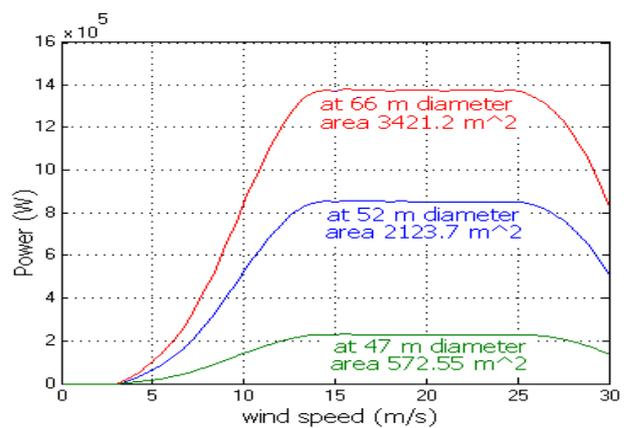
Figure 24 Effect of swept area on the generated power
