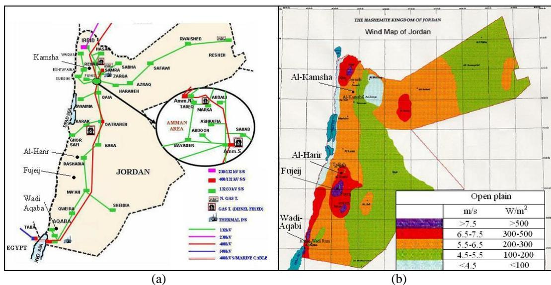
Figure 7 Jordan maps (a) Transmission lines and substations (Source: NEPCO), (b) Wind map resources (Ministry of Energy and Mineral Resources, 1998-2002)
