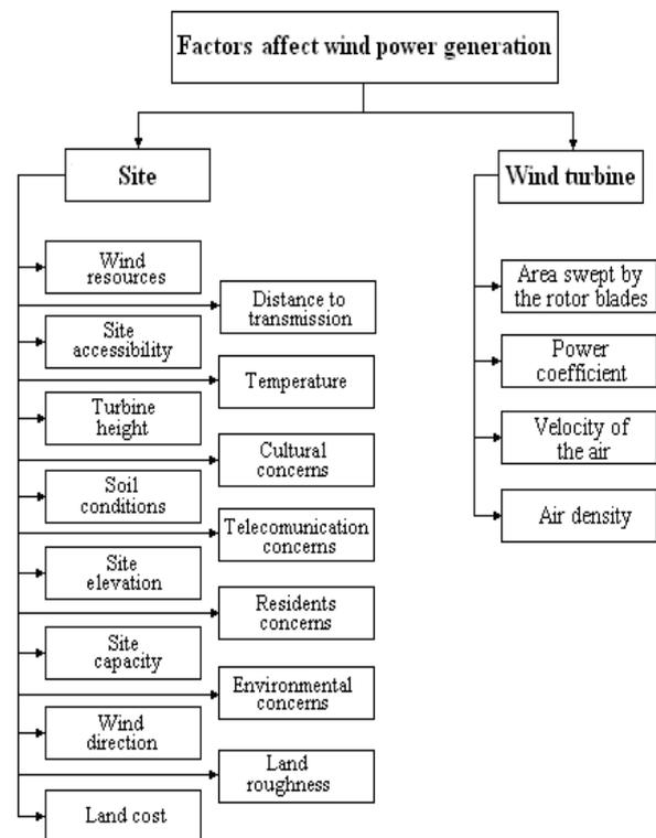
Figure 4 Classification of factors that affect wind power generation
