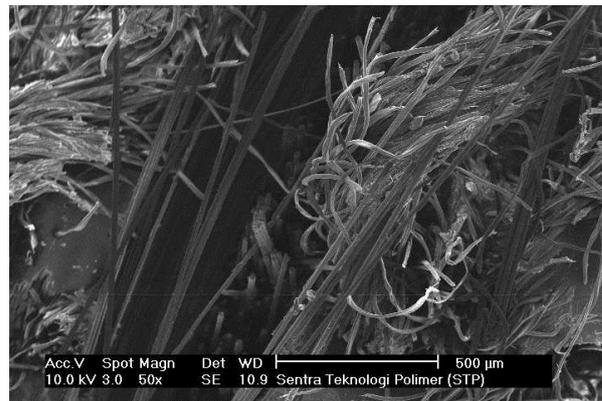
Figure 5 SEM micrographs of FGP (50x)
