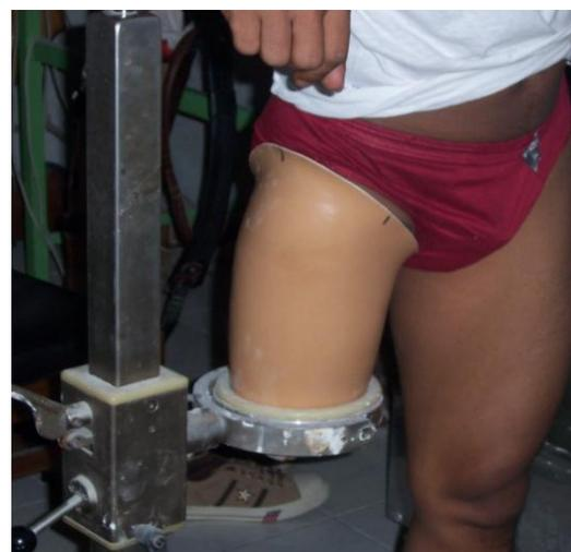
Figure 6 Static comfort test of socket prosthesis
