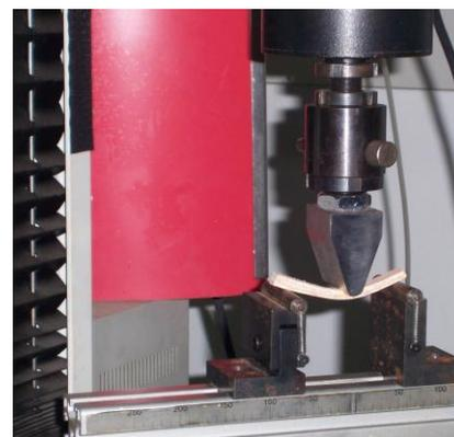
Figure 2 Flexural specimen test
