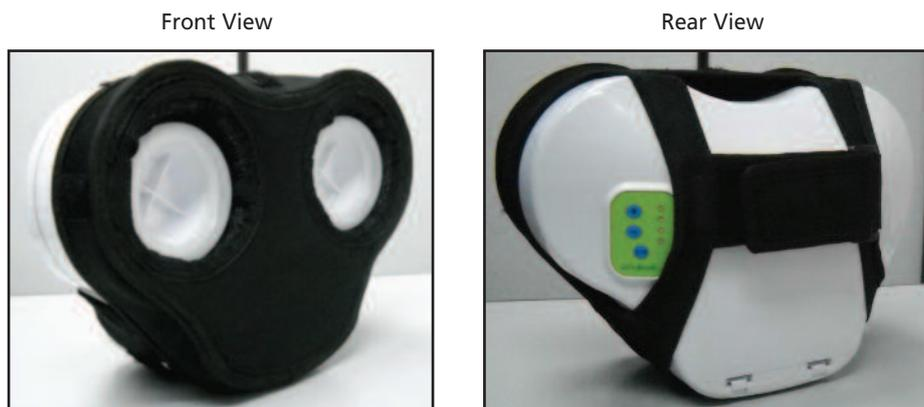
**Fig. 1 :** Illustration of the Percussor: It has a DC motor, Rechargeable battery pack, the cups have silicone pad with protein free (Neoprene) material cover. PCB (controls speed / Auto cut off)
