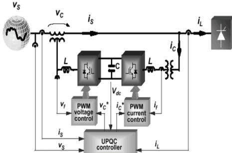
Figure 1: General configuration of Unified Series Shunt Compensator-USSC
