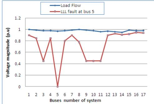
Figure 7: Voltage magnitudes of system buses at base case and During three phase fault at bus 5
