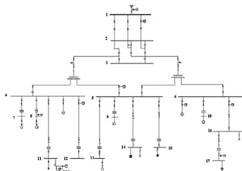
Figure 4: Topology of the distribution network of 15 nodes
