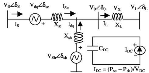
Figure 2: Equivalent circuit of USSC
