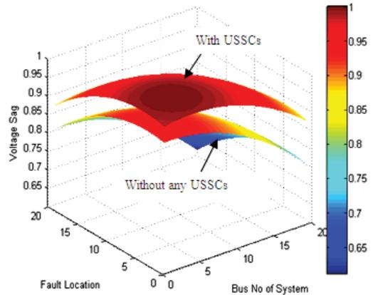
Figure 9: Improvement of sag distribution in terms of system buses due to three phase fault at various fault locations after USSCs placement
