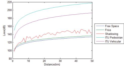
Figure 3: Path loss of different type of models
