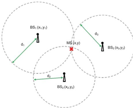
Figure 1: Multilateration with three base stations as the reference point to determine the mobile station.
