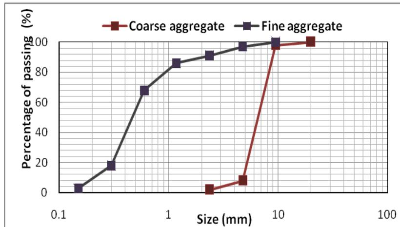
Figure 1 Grading curves of aggregates
