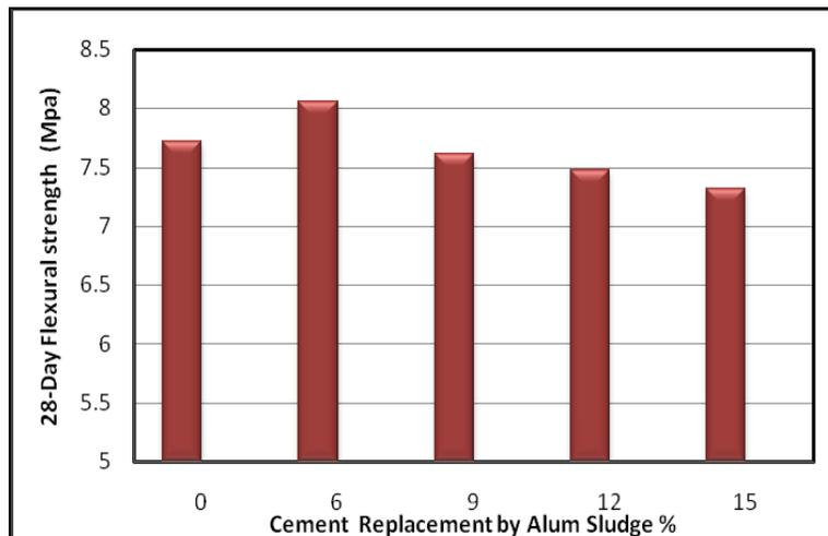
Figure 9 The effect of AS on flexural strength
