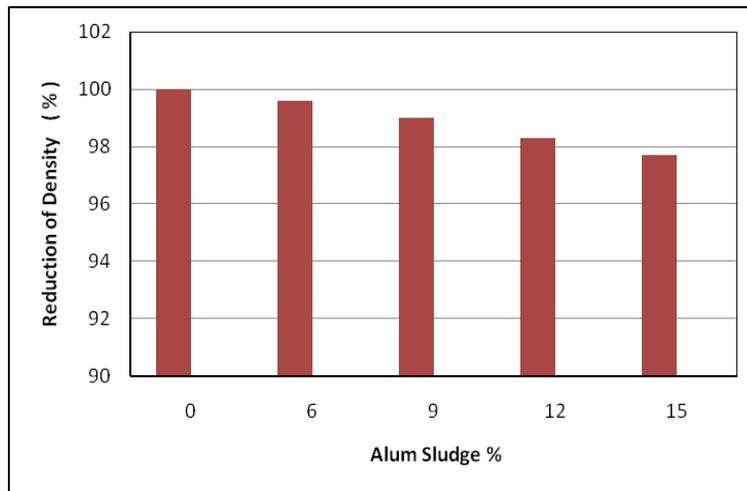
Figure 6 Effect of alum sludge on the reduction the density
