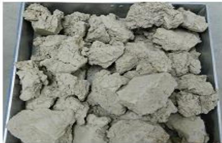
Figure 3 Alum sludge oven-dried at 110 °C
