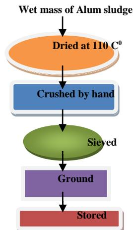
Figure 2 Schematic flow diagram of the preparation of the alum sludge sample
