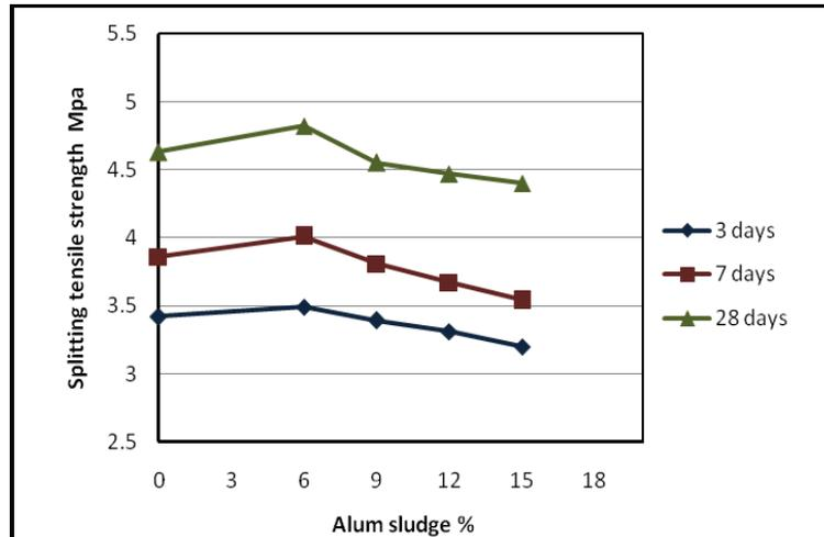
Figure 8 The effect of AS on splitting tensile strength
