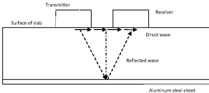
Figure 5 Direct and Reflected wave
