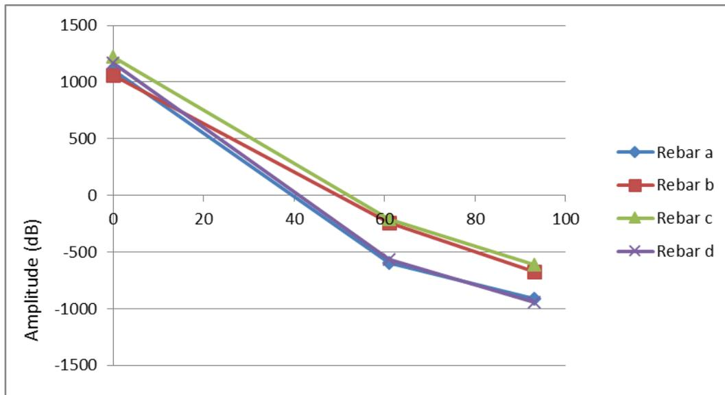
Figure 8 Amplitudes of GPR signals at reinforcing steels versus duration of immersion
