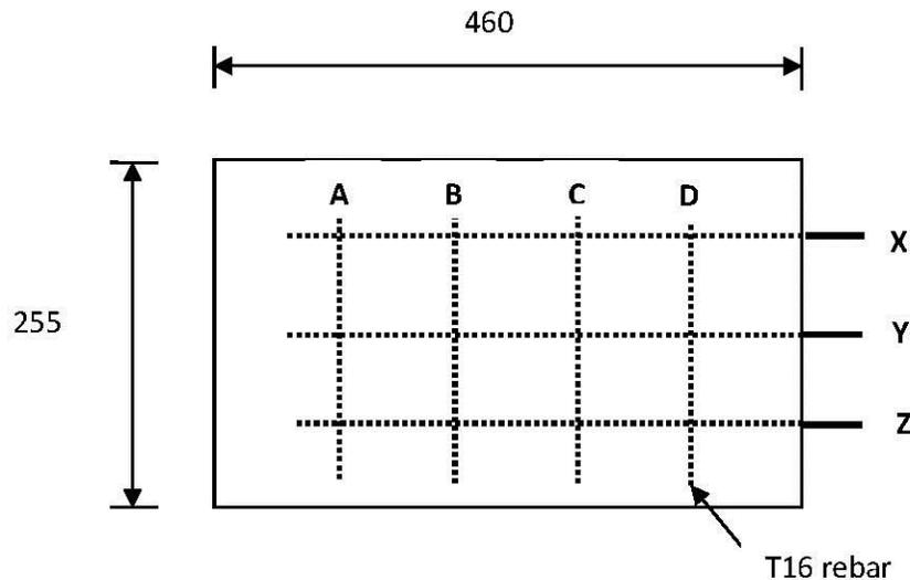
Figure 2 Schematic diagram of the reinforced concrete slab (All units are in mm)
