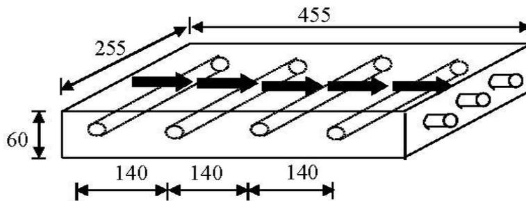
Figure 4 Direction of GPR scanning (All units are in mm)
