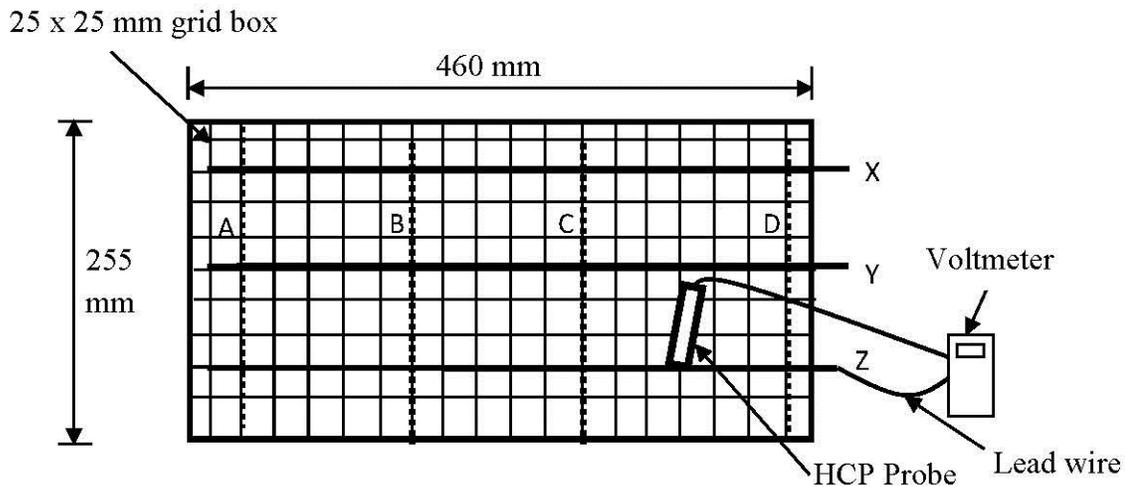
Figure 6 HCP difference measurement along the rebar using half cell probe
