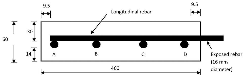
Figure 9 Dimension of side, top and bottom cover (All units are in mm)
