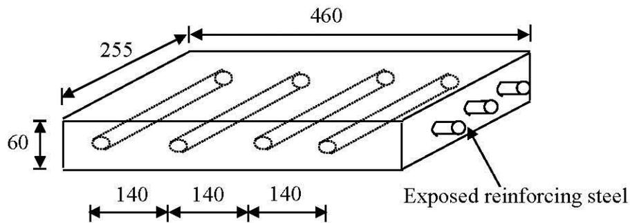
Figure 1 Isometric view of slab sample (All units are in mm)
