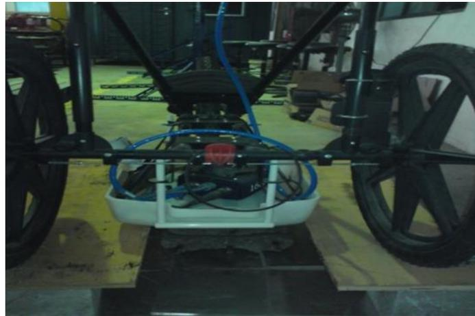
Figure 3 Ground Penetrating Radar equipment
