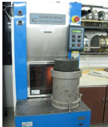
**Figure 2** Superpave Gyrotory Compactor (SGC)
