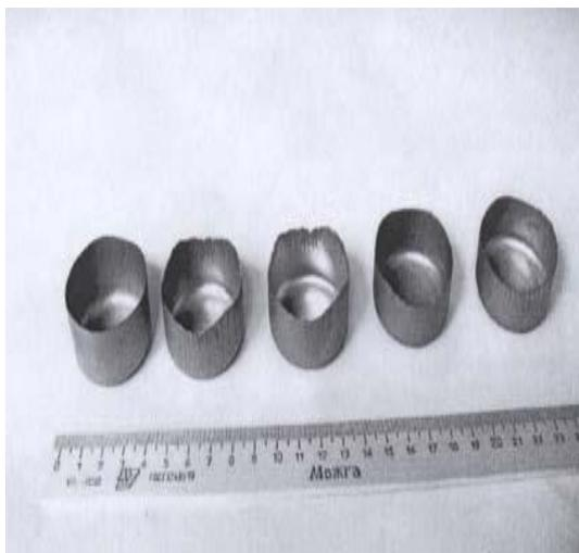
Figure 7. Cylindrical Specimens Fabricated by Means of Deep Drawing
