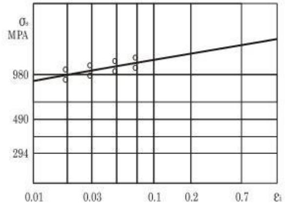
Figure 5. Dependence of  $\sigma_s$  and  $\varepsilon_i$  in Logarithm Coordinates
