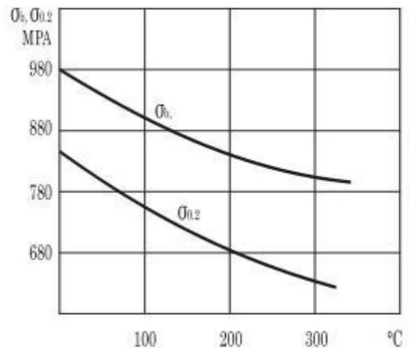
Figure 6. Variation of Mechanical Properties of Molybdenum by Temperature
