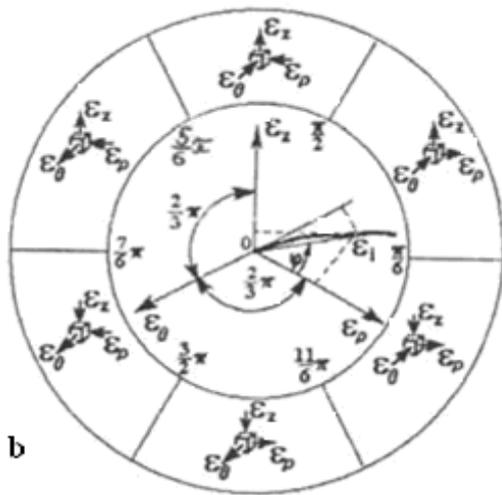
Figure 3. Stress (a) and Strain (b) States of the Axisymmetric Shell (Nazaryan and Konstantinov 1999)
