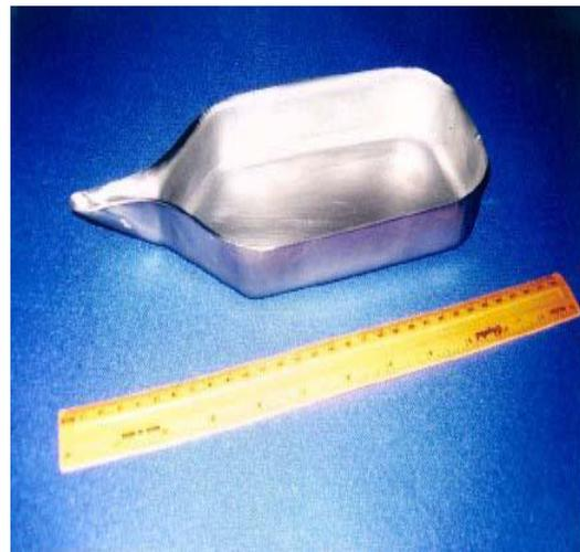
Figure 8. The Boat-Shaped Container Fabricated by Means of Deep Drawing.
