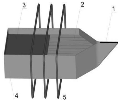
Figure 1. A Schematic of the Bagdasarov Method (1 - Seed, 2 - Crystal, 3 - Melt, 4 - Container, 5 - Heater)
