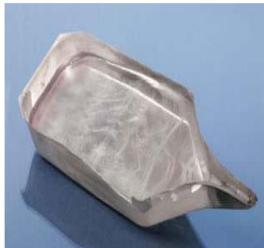
Figure 9. The Container with Growth Single Crystal.
