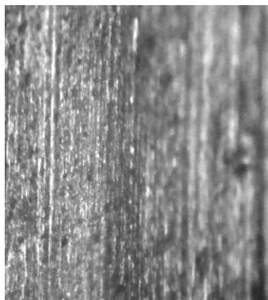
Figure 3: Wear scar of Al 6063-O for 3 N applied load
