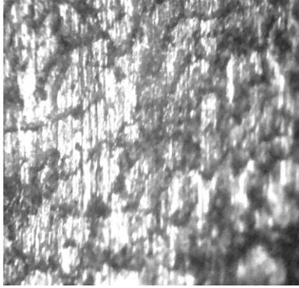
Figure 4: Wear scar of cast Al A 356.0 (soft) for 3 N applied load
