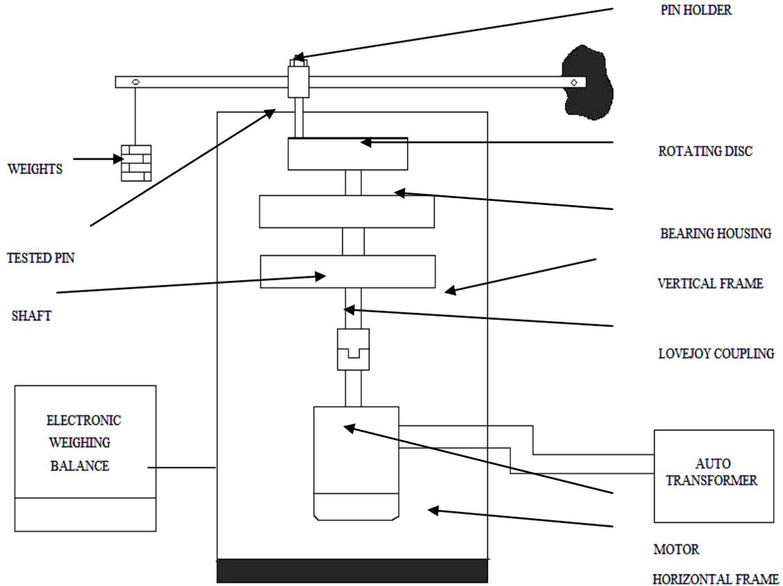
Figure 1: Pin on disc wear test apparatus
