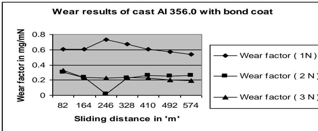
Figure 2 : Wear factor in  $10^{-3}$  mg/Nm as a function of sliding distance and applied load
