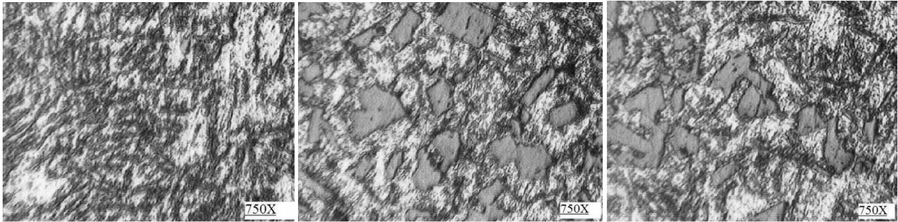
Figure 4 Microstructures at outer, middle and inner surfaces for rotational speed 200 rpm
