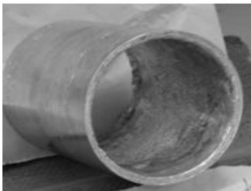
Figure 8 b Centrifugal Castings (size  $\varnothing$  80, 120mm long) produced at 600 rpm
