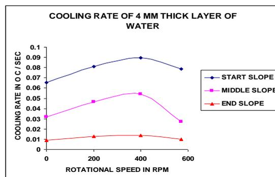
Figure 3 Cooling rate at different rotational speeds
