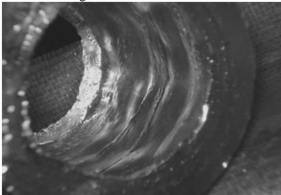
Figure 8 a Centrifugal Castings (size  $\varnothing$  80, 120mm long) produced at a) 400 rpm
