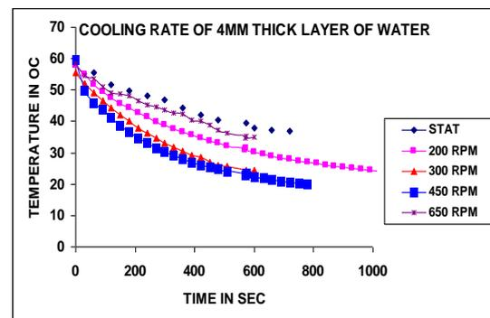
Figure 2 Temperature variation of the water at different intervals of time
