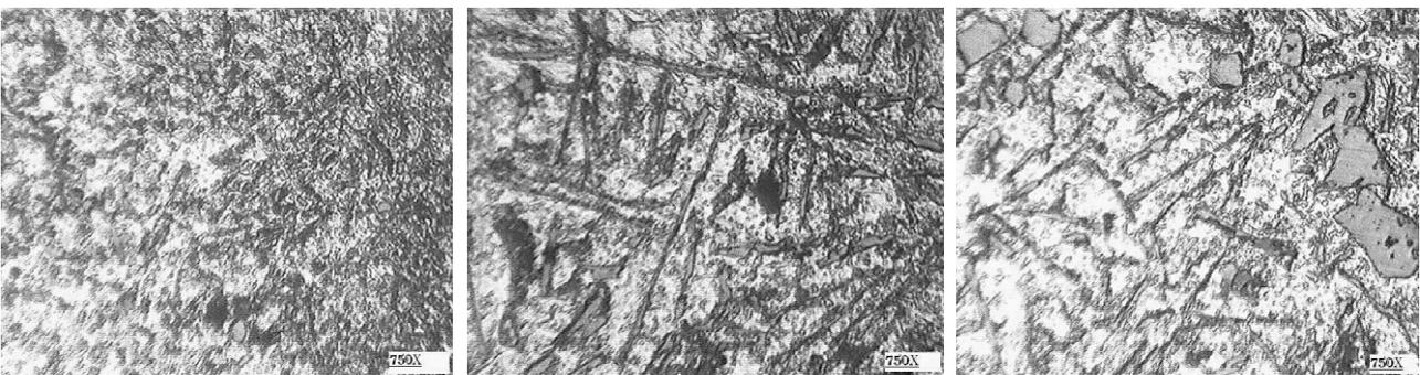
Figure 7 Microstructures at outer, middle and inner surfaces for rotational speed 800rpm
