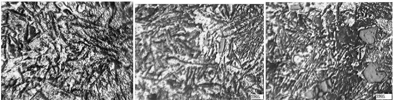
Figure 5 Microstructures at outer, middle and inner surfaces for rotational speed 400 rpm
