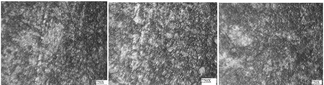
Figure 6 Microstructures at outer, middle and inner surfaces for rotational speed 600 rpm
