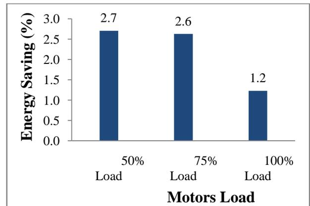
Figure 5 Energy saving percentage (%) by high efficient motors
