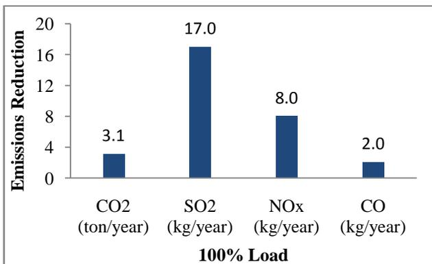
Figure 8 Total annual emissions reduction by high efficient motors at 100% load
