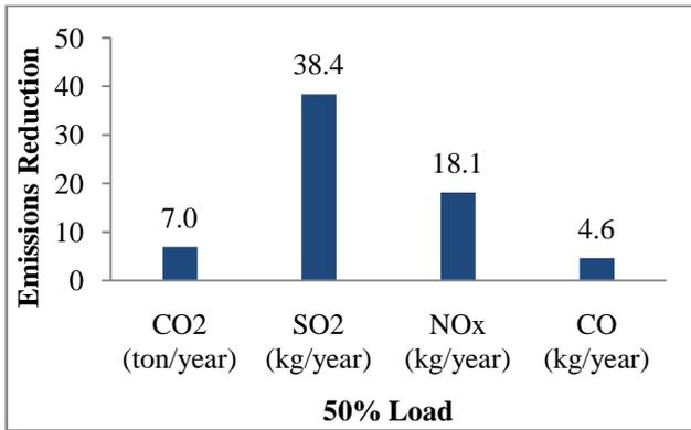
Figure 6 Total annual emissions reduction by high efficient motors at 50% loads
