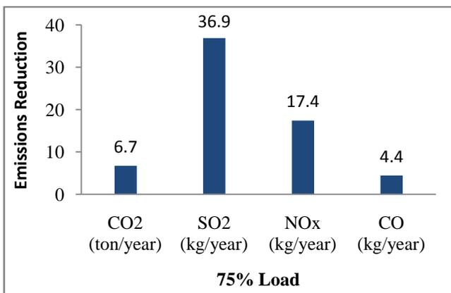
Figure 7 Total annual emissions reduction by high efficient motors at 75% load
