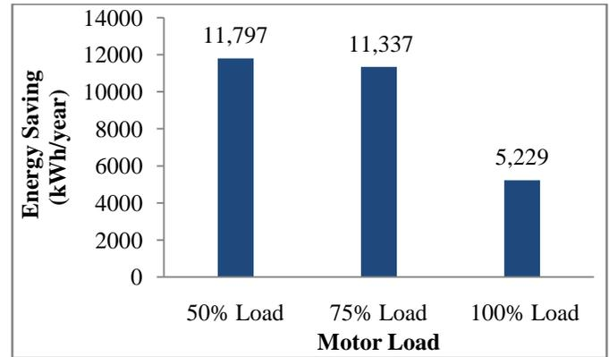
Figure 4 Total annual energy saving (kWh/year) by high efficient motors
