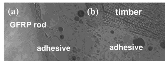
Figure 10: Optical micrographs of failed pull-out specimens for Timberset: (a) Joint between the GFRP rod and adhesive and (b) Joint between adhesive and timber.
