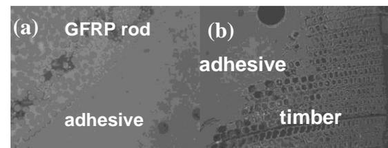
Figure 9: Optical micrographs of failed pull-out specimens for Albipox: (a) Joint between the GFRP rod and adhesive and (b) Joint between adhesive and timber.
