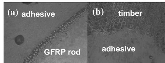
Figure 8: Optical micrographs of failed pull-out specimens for CB10TSS: (a) Joint between the GFRP rod and adhesive and (b) Joint between adhesive and timber.
