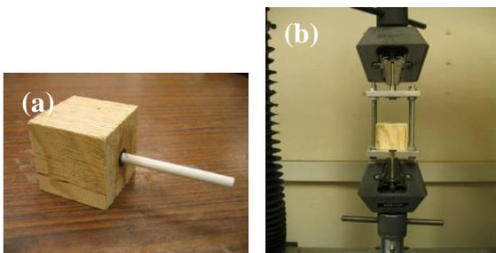
Figure 3: (a) Single-ended pull-out test specimen and (b) Experimental set-up for pull out test.
