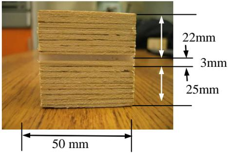
Figure 2: Block shear test specimen.
