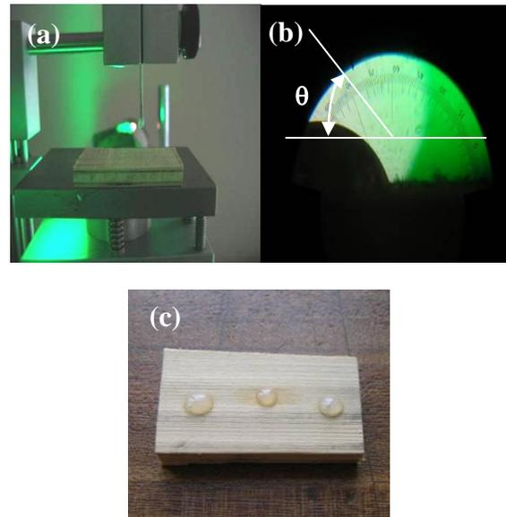
Figure 1: Showing; (a) Sessile droplets of CB10TSS adhesive, (b) measurement of contact angle,  $\theta$ , and (c) LVL blocks with droplets of adhesives.
