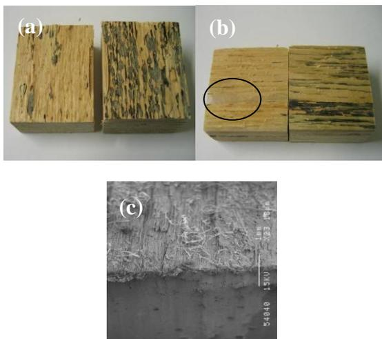
Figure 6: Failure mode of block shear sample: (a) for CB10TSS: cohesive timber failure, (b) for Nanopox: crack propagation in the timber with small part failed at the adhesive-timber interface (indicated by the marked
