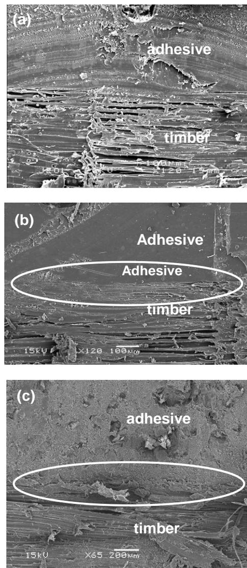
Figure 7: SEM micrographs of the sectioned surface of block shear specimens of (a) CB10TSS, x 120, (b) Albipox, x 120, the marked circle shows smooth bond-
