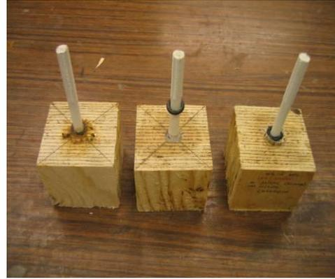
Figure 5: Different modes of failure; (a) timber failure (t), (b) rod/adhesive failure (ra) and (c) timber/adhesive failure (ta).
