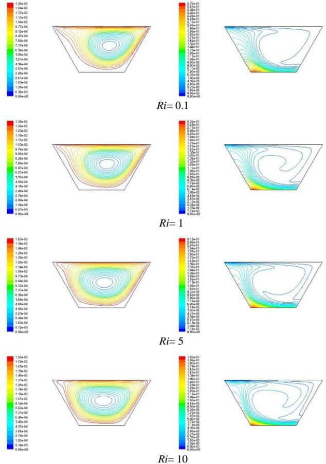
Figure 7: Contours of Streamlines and isotherms at  $Re=400$ ,  $A=1.0$  and  $\gamma=60^\circ$
