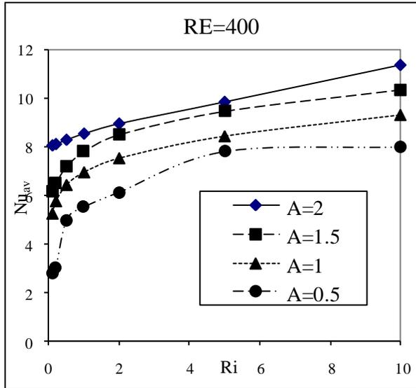
Figure 19: Variation of  $Nu_{av}$  with  $Ri$  at  $Re=400$  and  $\Phi=0^\circ$
