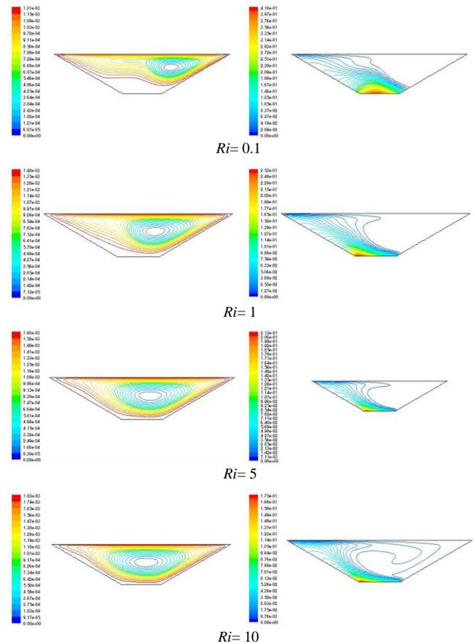
Figure 5: Contours of Streamlines and isotherms at  $Re=400$ ,  $A=1.0$  and  $\gamma=30^\circ$
