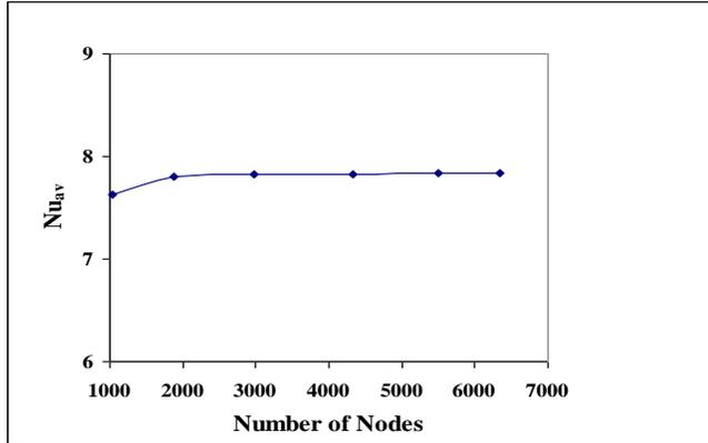
Figure 3: Grid sensitivity test for Trapezoidal cavity at  $Ri=1.0$ ,  $Re=400$  and  $A=1$ .
