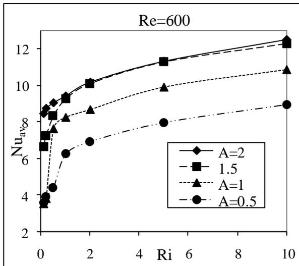
Figure 20: Variation of  $Nu_{av}$  with  $Ri$  at  $Re=600$  and  $\Phi=0^\circ$
