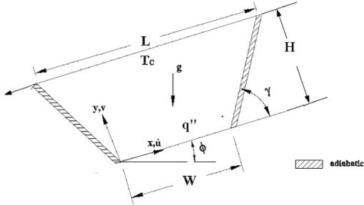
Figure 2: Schematic diagram of the physical system considering aiding flow condition
