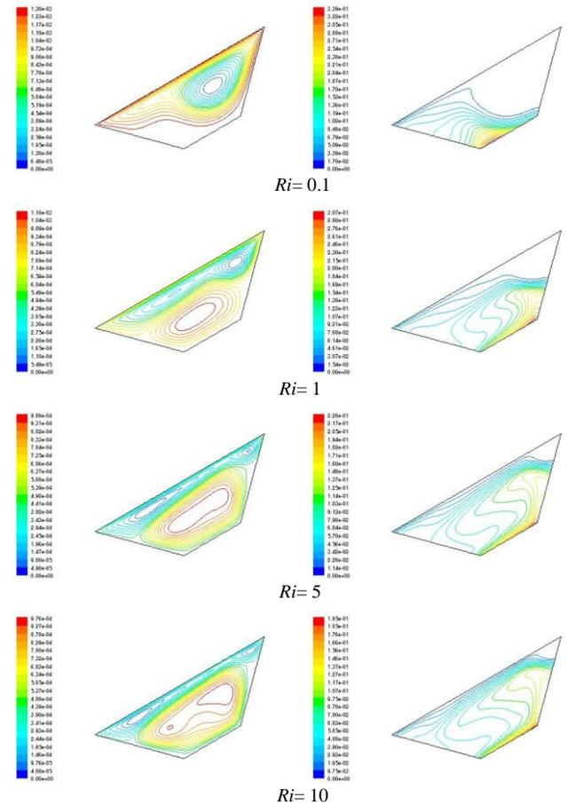
Figure 11: Contours of Streamlines and isotherms at  $Re=400$ ,  $A=1$  and  $\Phi=30^\circ$ , Opposing Flow
