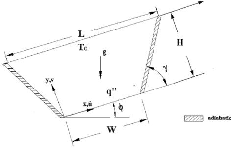
Figure 1: Schematic diagram of the physical system considering opposing flow condition
