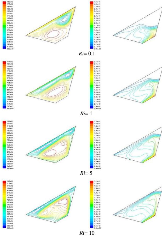
Figure 12: Contours of Streamlines and isotherms at  $Re=400$ ,  $A=1.5$  and  $\Phi=30^\circ$ , Opposing Flow
