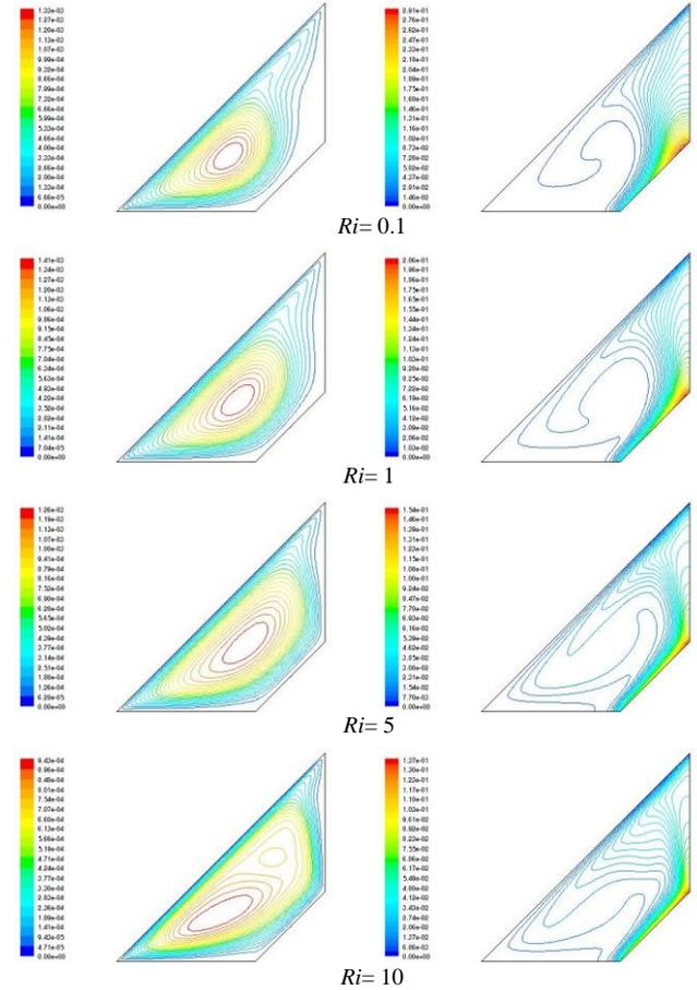
Figure 13: Contours of Streamlines and isotherms at  $Re=400$ ,  $A=1$  and  $\Phi=45^\circ$ , Aiding Flow
