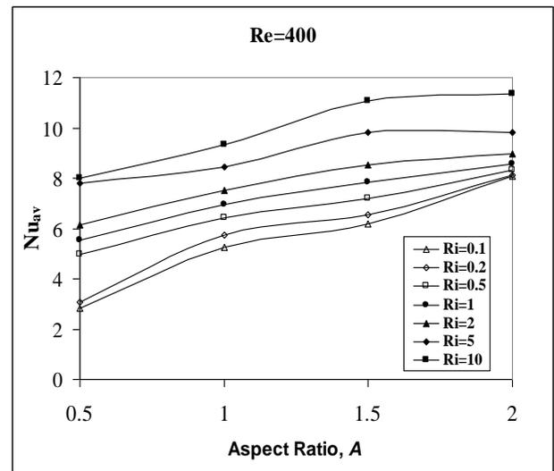
Figure 21: Variation of  $Nu_{av}$  with  $A$  at  $Re=400$  and  $\Phi=0^\circ$
