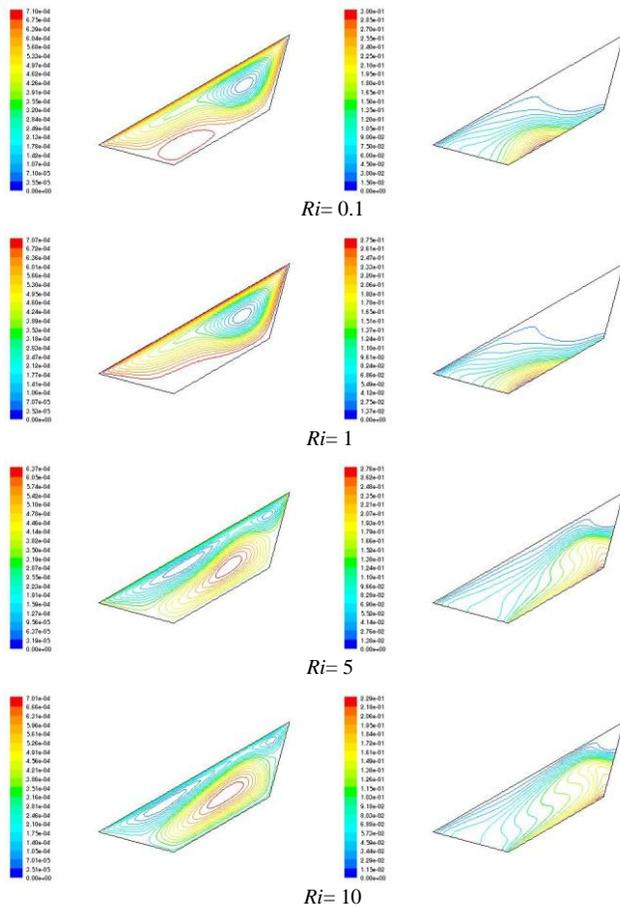
Figure 10: Contours of Streamlines and isotherms at  $Re=400$ ,  $A=0.5$  and  $\Phi=30^\circ$ , Opposing Flow
