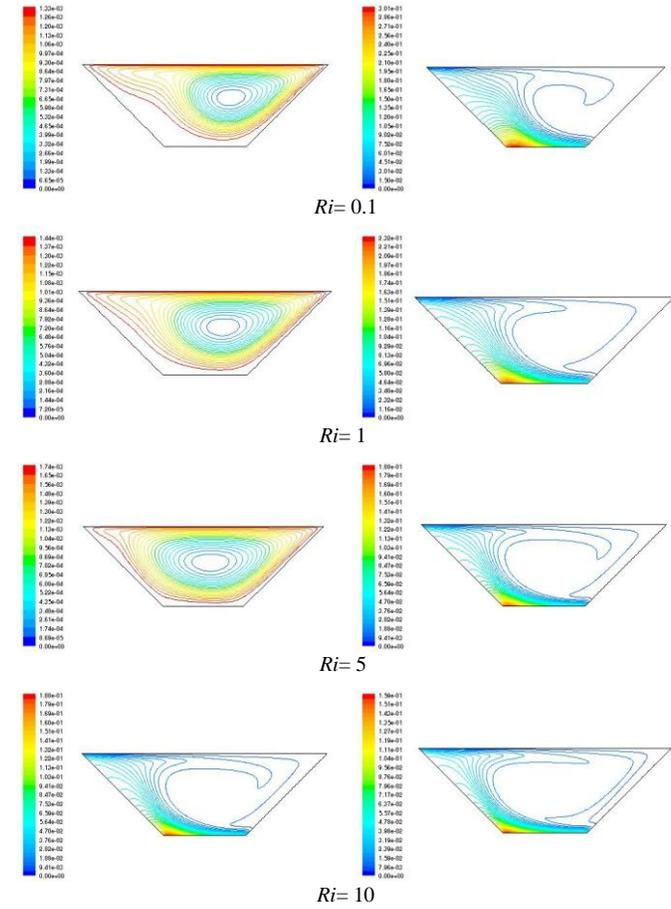
Figure 6: Contours of Streamlines and isotherms at  $Re=400$ ,  $A=1.0$  and  $\gamma=45^\circ$
