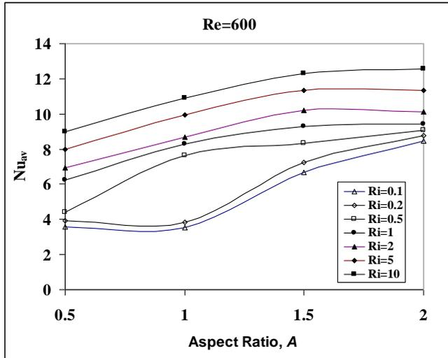
Figure 22: Variation of  $Nu_{av}$  with  $A$  at  $Re=600$  and  $\Phi=0^\circ$
