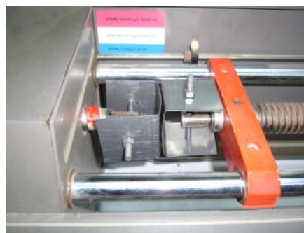
Figure 3 (b) Sample loaded in tensometer
