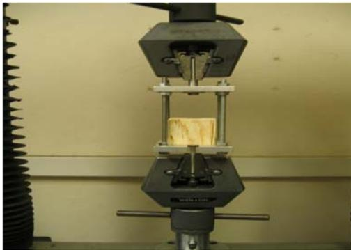
Figure 3: Experimental set-up for pull out test.
