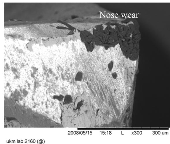
Fig. 1. Wear on the flank face when machining at cutting speed of 180 m/min, feed rate of 0.1 mm/tooth and depth of cut of 0.3 mm
