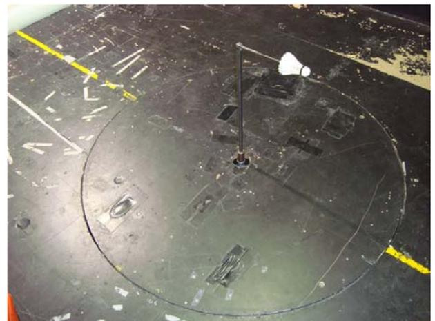
Figure 7(d) A complete setup (sting & shuttlecock)
