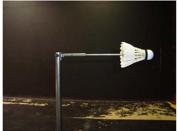
Figure 7(b) Sting with shuttlecock (side view)
