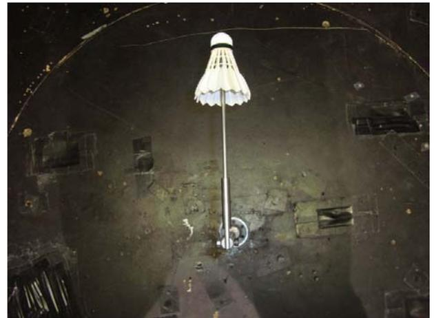
Figure 7(c) Sting with shuttlecock (top view)
