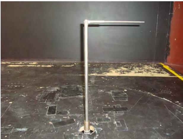
Figure 7(a) Experimental setup of the sting on a six component force sensor
