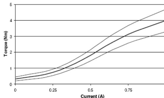
Figure 2 Torque (N m) vs. current I in the coil
