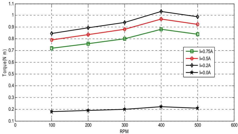
Figure 8 The torque ( $T$ ) vs. rotary speed ( $\omega$ ) at various field strengths:  $I = 0.0, 0.20, 0.50, 0.75$  A.
