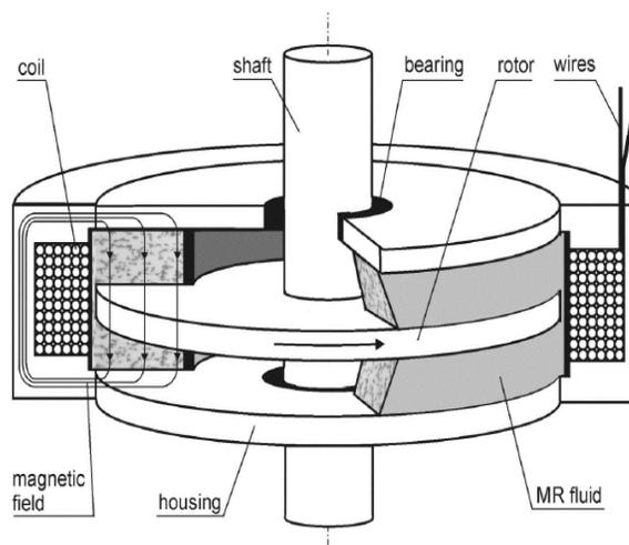
Figure 3 Schematic diagram of MR rotary brake.
