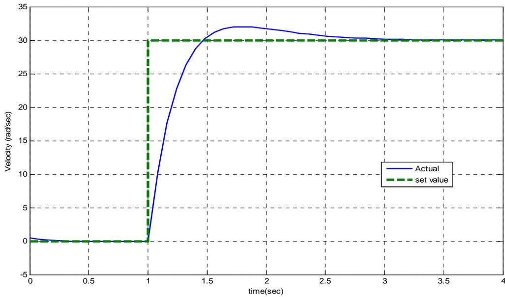
Figure 7 Torque control system response to the repeated sequence change of preset velocity for the system with a MR brake
