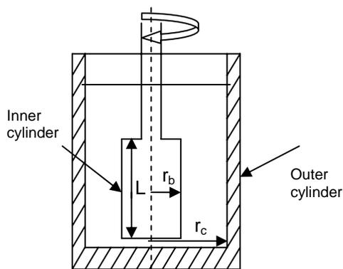
Figure 1 Schematic diagram of rotary damper.
