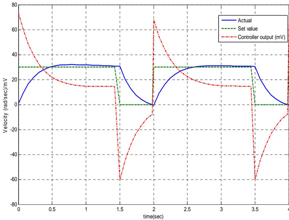
Figure 6 Torque control system response to the repeated sequence change of preset velocity for the system with a MR brake
