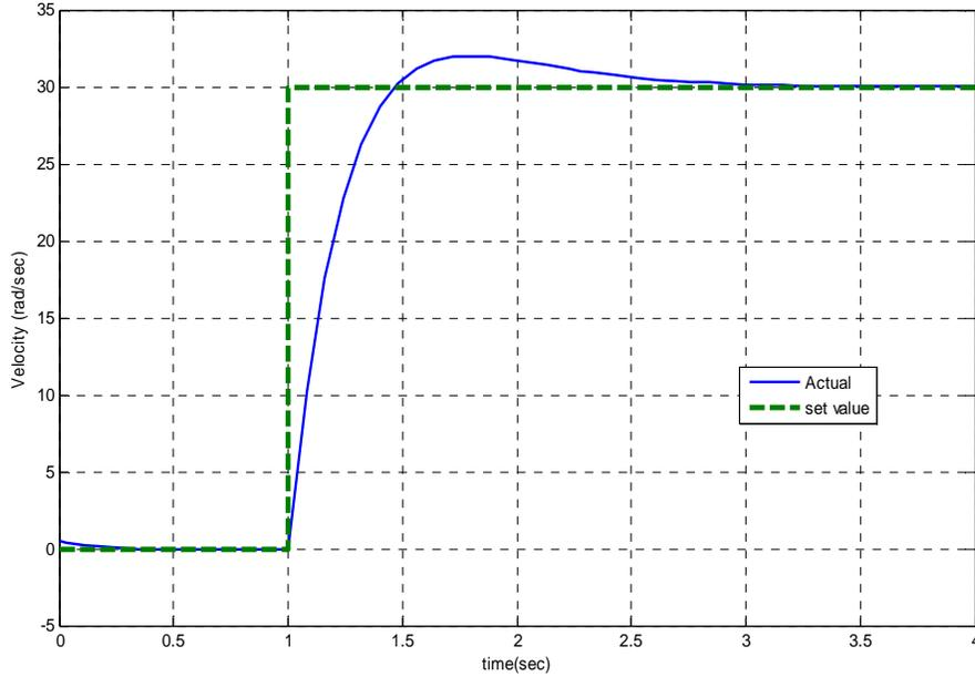
Figure 5 Torque control system response to the step change of preset velocity for the system with a MR brake,
