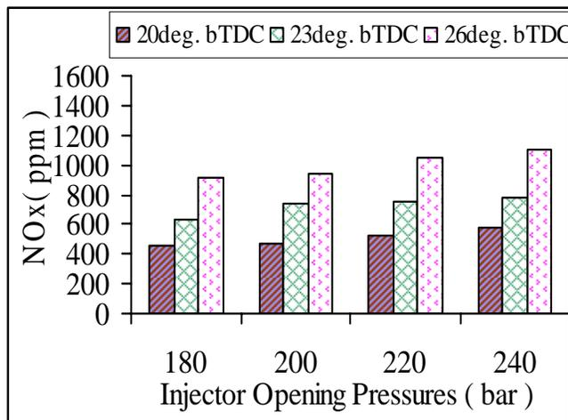
Figure 19 Variation of NO<sub>x</sub> with different IOPs of B20 fuel at full load conditions.
