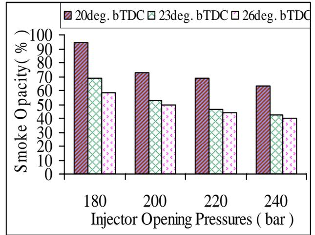
Figure 16 Variation of smoke opacity with different IOPs of B100 fuel at full load conditions.
