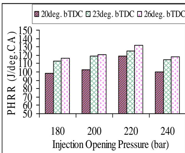
Figure 27 Variation of peak heat release rate with different IOPs of B20 fuel at full load conditions.
