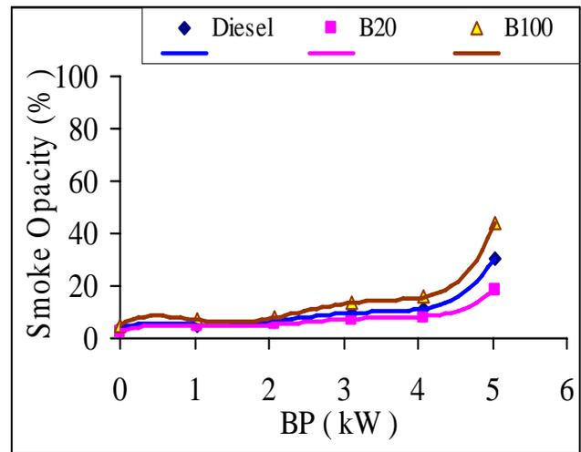
Figure 17 Variation of smoke opacity with BP of diesel, B20 and B100 fuel at IOP 220bar and IT 26deg. bTDC.
