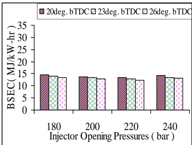
Figure 6 Variation of BSEC with different IOPs of diesel fuel at full load conditions.
