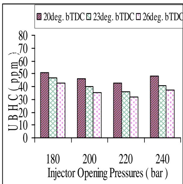
Figure 11 Variation of UBHC with different IOPs of B20 fuel at full load conditions.
