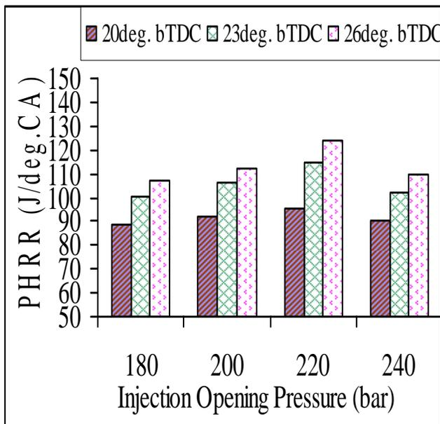
Figure 26 Variation of peak heat release rate with different IOPs of diesel fuel at full load conditions.
