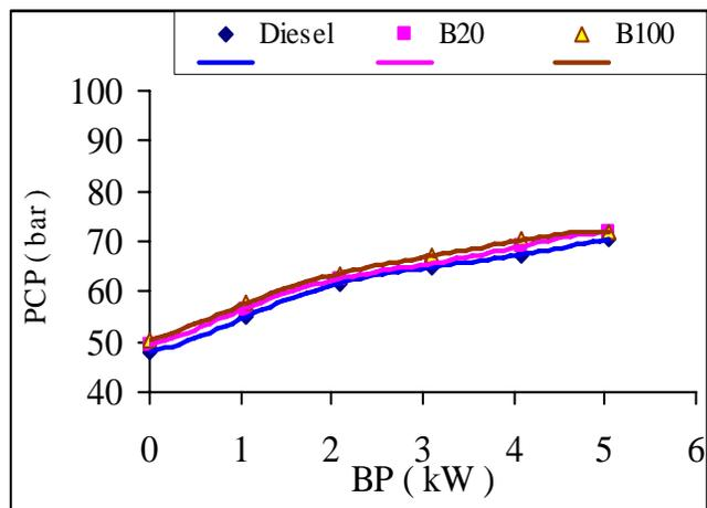
Figure 25 Variation of peak cylinder pressure with BP of diesel, B20 and B100 fuel at IOP 220bar and IT 26deg. bTDC.
