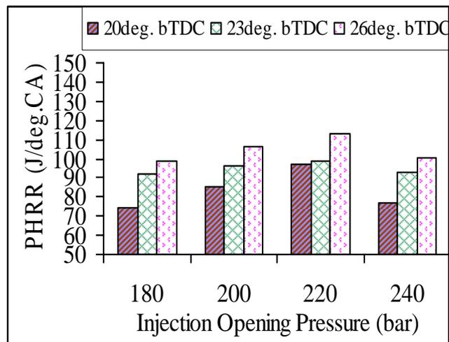
Figure 28 Variation of peak heat release rate with different IOPs of B100 fuel at full load conditions.
