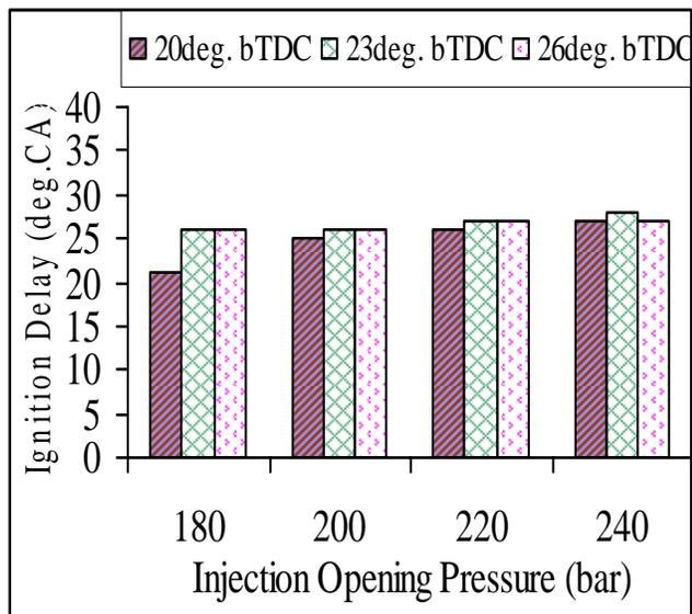
Figure 31 Variation of ignition delay with different IOPs of B20 fuel at full load conditions.
