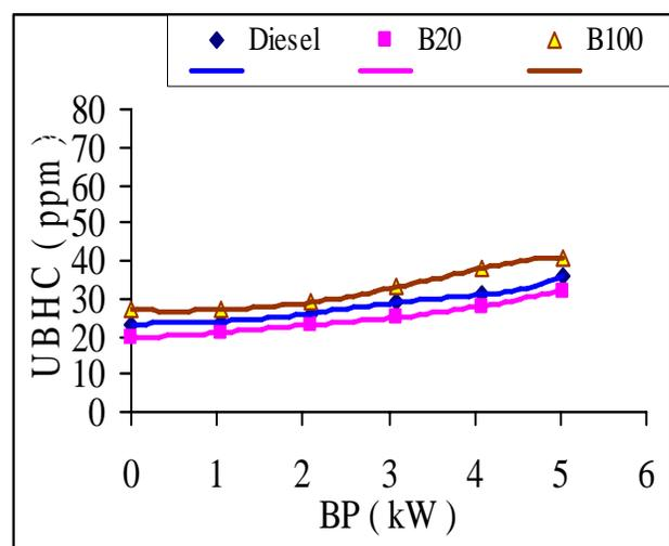
Figure 13 Variation of UBHC with BP of diesel, B20 and B100 fuel at IOP 220bar and IT 26deg. bTDC.
