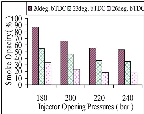
Figure 15 Variation of smoke opacity with different IOPs of B20 fuel at full load conditions.
