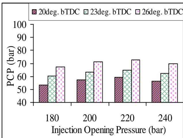
Figure 23 Variation of peak cylinder pressure with different IOPs of B20 fuel at full load conditions.
