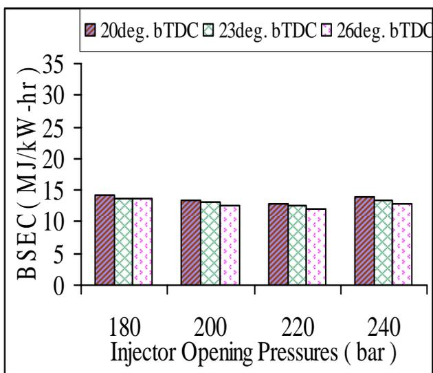
Figure 7 Variation of BSEC with different IOPs of B20 fuel at full load conditions.
