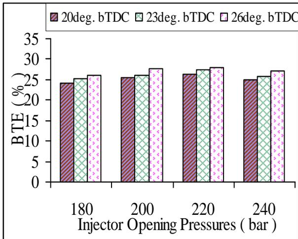
Figure 4 Variation of BTE with different IOPs of B100 at fuel full load conditions.
