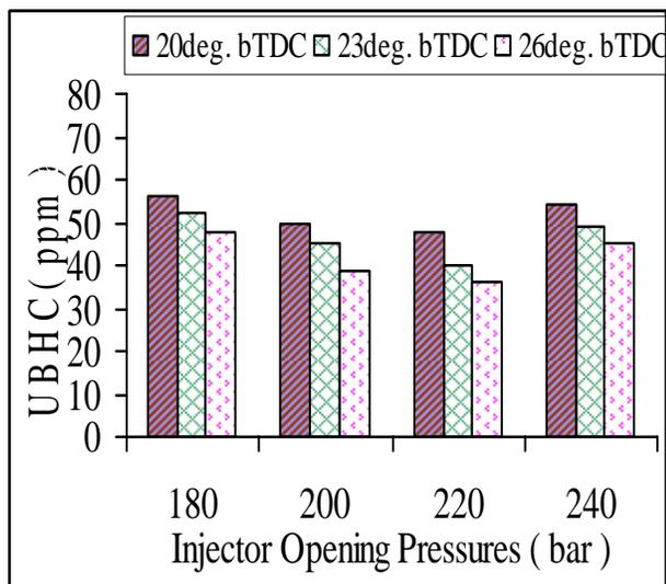
Figure 10 Variation of UBHC with different IOPs of diesel fuel at full load conditions.
