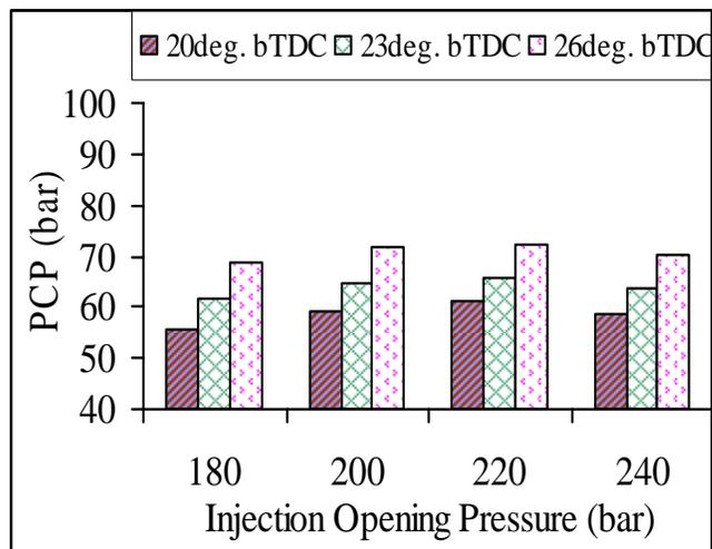
Figure 24 Variation of peak cylinder pressure with different IOPs of B20 fuel at full load conditions.
