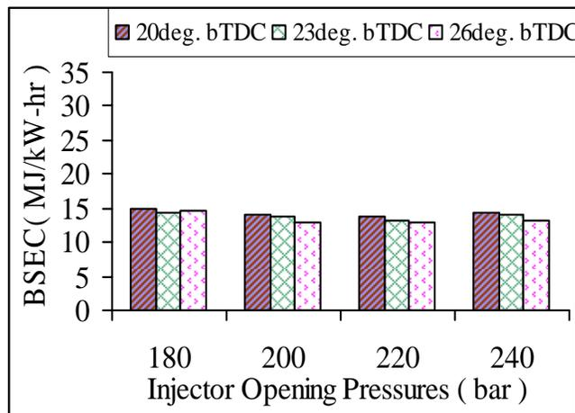
Figure 8 Variation of BSEC with different IOPs of B100 fuel at full load conditions.
