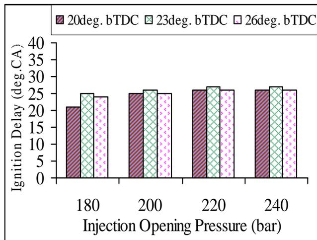
Figure 32 Variation of ignition delay with different IOPs of B100 fuel at full load conditions.
