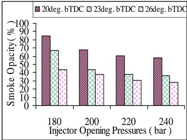
Figure 14 Variation of smoke opacity with different IOPs of diesel fuel at full load conditions.
