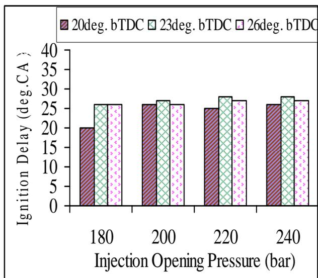
Figure 30 Variation of ignition delay with different IOPs of diesel fuel at full load conditions.
