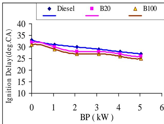
Figure 33 Variation of Ignition delay with BP of diesel, B20 and B100 fuel at IOP 220bar and IT 26deg. bTDC.
