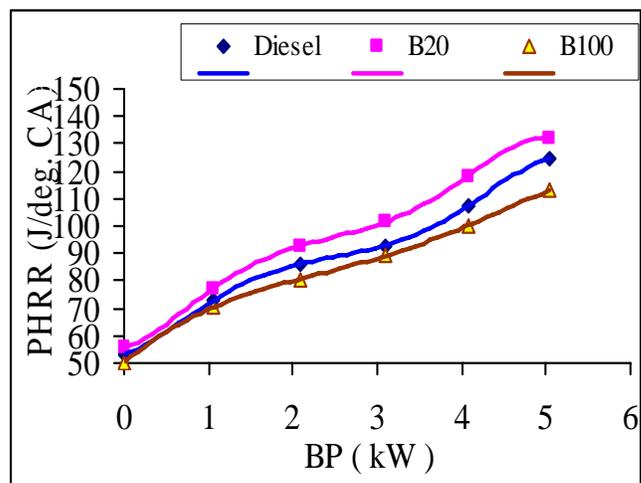
Figure 29 Variation of peak heat release rate with BP of diesel, B20 and B100 fuel at IOP 220bar and IT 26deg. bTDC.
