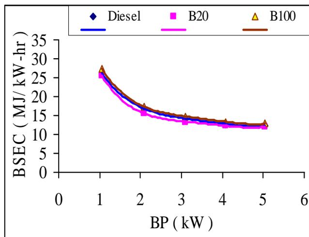
Figure 9 Variation of BSEC with BP of diesel, B20 and B100 fuel at IOP 220bar and IT 26deg. bTDC.
