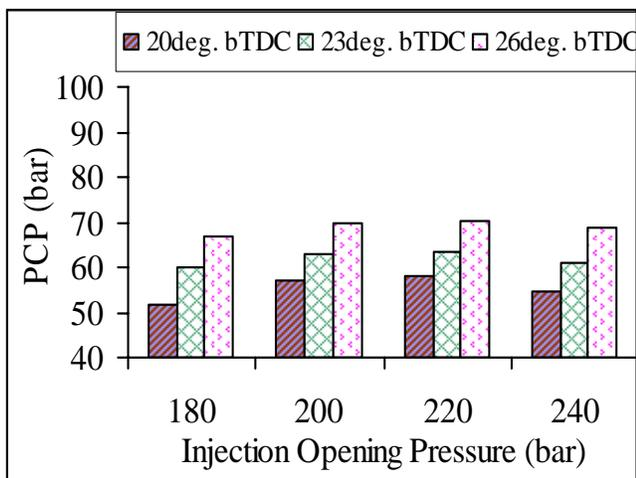
Figure 22 Variation of peak cylinder pressure with different IOPs of diesel fuel at full load conditions.
