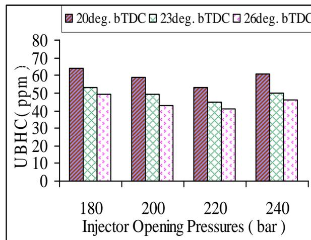
Figure 12 Variation of UBHC with different IOPs of B100 fuel at full load conditions.
