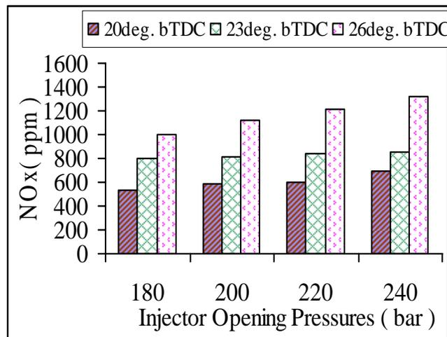
Figure 20 Variation of NO<sub>x</sub> with different IOPs of B100 fuel at full load conditions.
