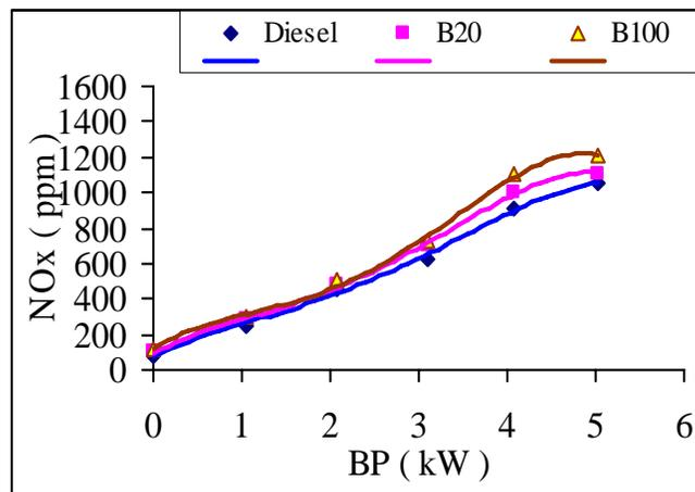
Figure 21 Variation of NO<sub>x</sub> with BP of diesel, B20 and B100 fuel at IOP 220bar and IT 26deg. bTDC.
