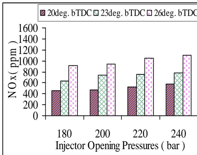
Figure 18 Variation of NO<sub>x</sub> with different IOPs of diesel fuel at full load conditions.
