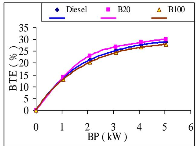
Figure 5 Variation of BTE with BP of diesel, B20 and B100 fuel at IOP 220bar and IT 26deg. bTDC.
