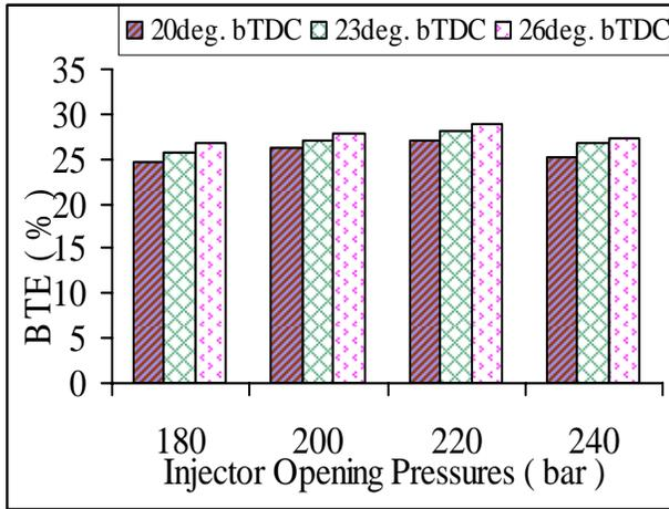
Figure 2 Variation of BTE with different IOPs of diesel fuel at full load conditions.
