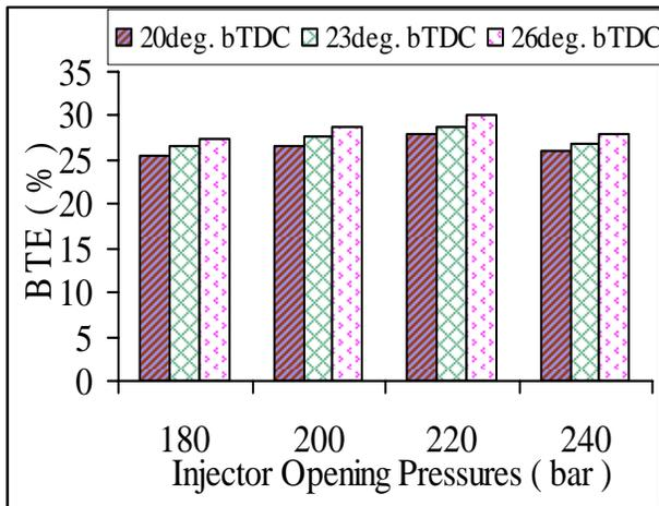
Figure 3 Variation of BTE with different IOPs of B20 fuel at full load conditions.
