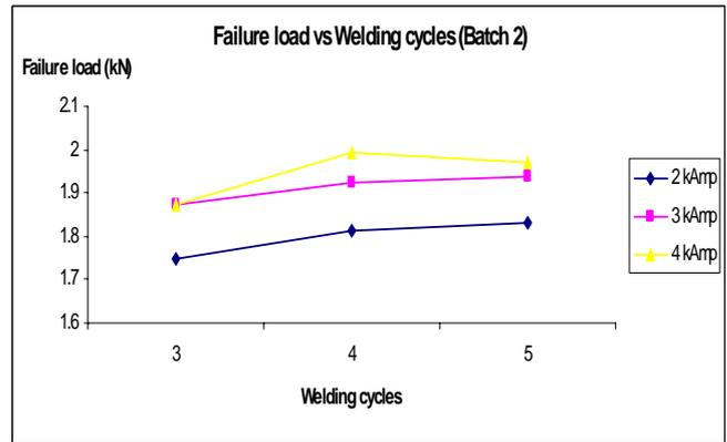
Fig 7. Correlation between failure load and welding cycles (Batch 2)
