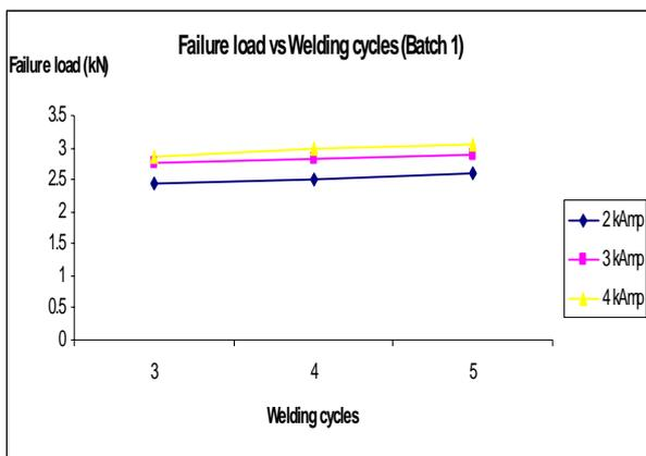
Fig. 6 Correlation between failure load and welding cycles (Batch 1)
