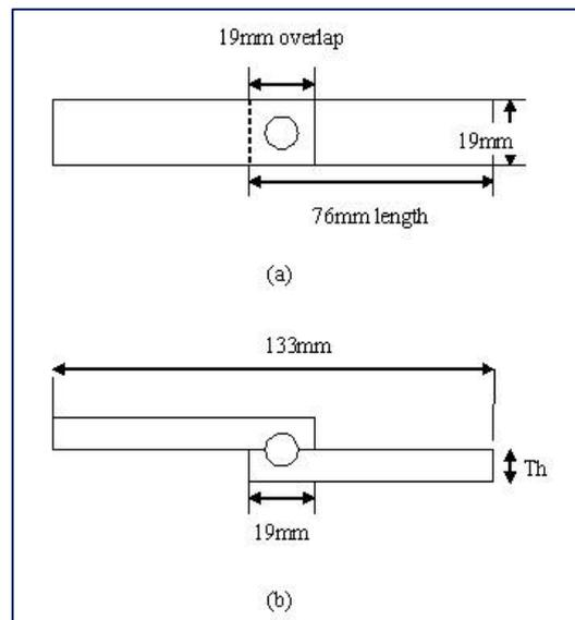
Fig.1 Standard dimension for tensile shear testing (a) Plan view, (b) Side view
