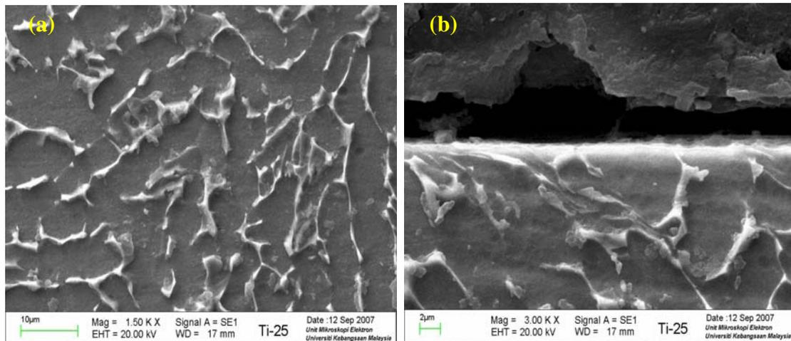
Figure 4: Microstructure below Machined Surface (a) and White Layer on Top Machined Surface (b) after machining with Coated Cemented Insert at a Cutting Speed of 95 m/min, a Feed Rate of 0.35 mm/rev and a Depth of Cut 0.10 mm
