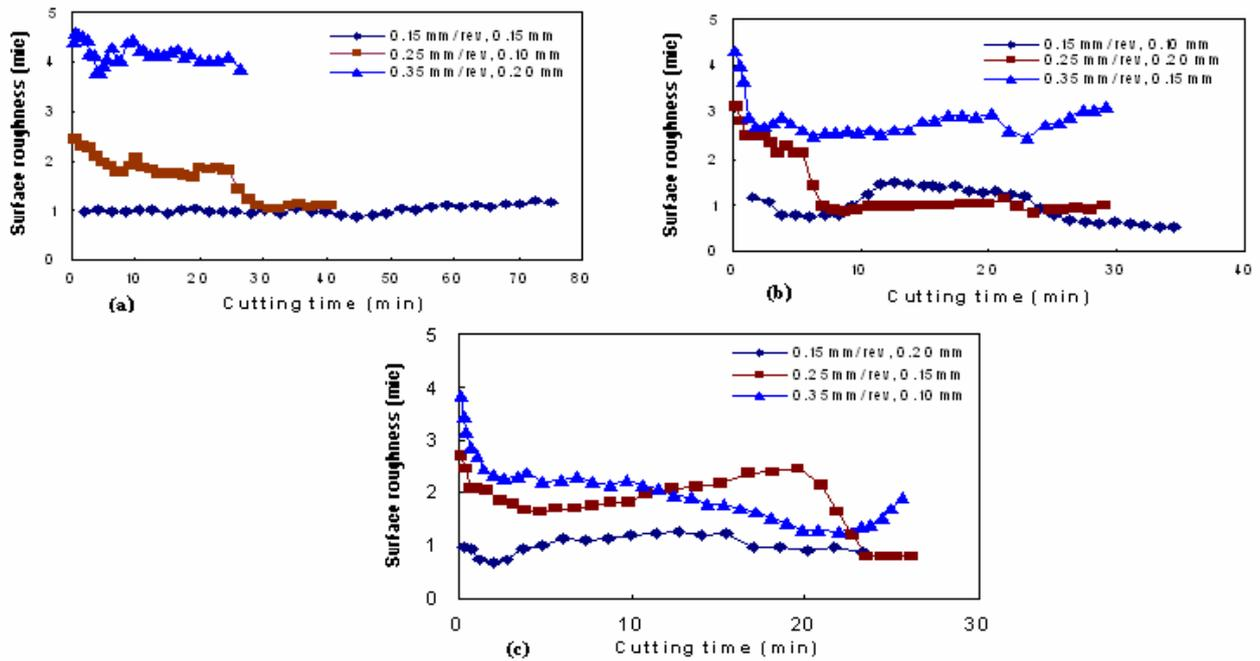
Figure 1: Surface Roughness Values Recorded at Cutting Speed of (a) 55 m/min, (b) 75 m/min and (c) 95 m/min
