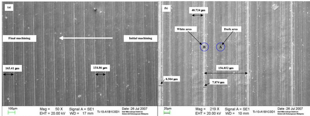
Figure 2: Surface Generated when Machining with Coated Cemented Carbide Insert Under Dry Machining (a) 50x Magnification and (b) 219x Magnification.
