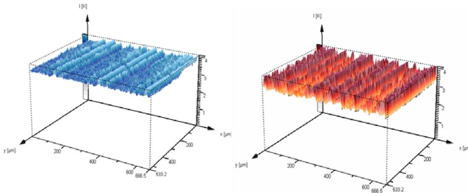
Figure 5. Surface Topography of Machined Surface after Machining of Titanium Alloys Ti-6Al-4V ELI by Using Coated Cemented Carbide Tools; (a) at cutting speed of 55 m/min and feed rate of 0.25 mm/rev (b) at cutting speed of 95 m/min and feed rate of 0.35 mm/rev
