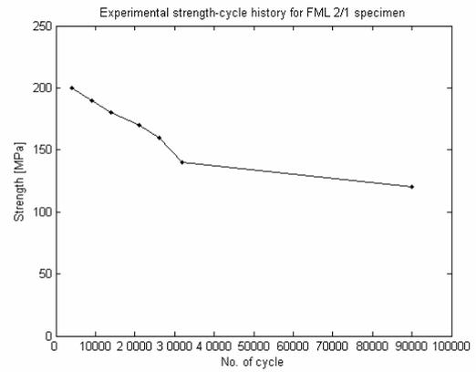
Fig. 3 S-N curve which was obtained from the experiment
