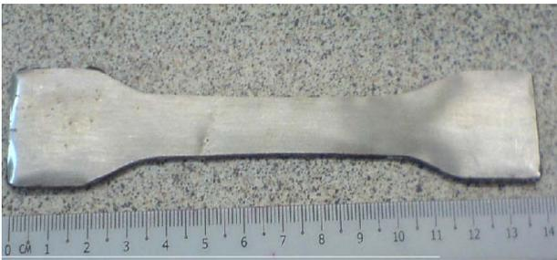
Figure 1: The geometry and shape of FML specimen used in this study
