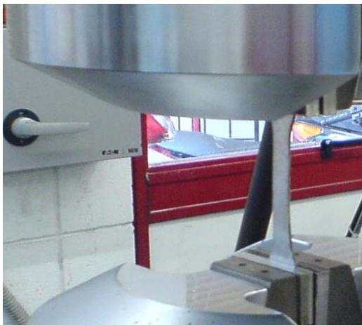
Figure 2: A FML specimen fitted at the fatigue machine
