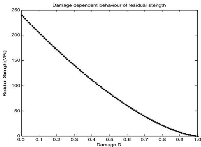
Figure 5: Damage dependent behavior of residual strength
