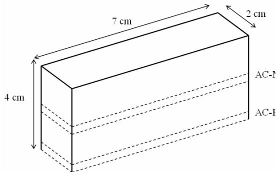
Figure 1: Schematic of the sectioned AC-M and AC-B specimens
