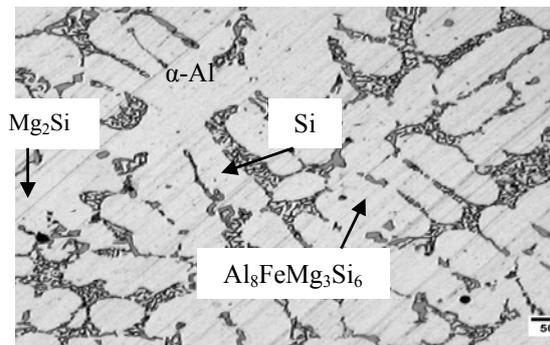
Figure 3: Optical micrographs of superheated as-cast AC-B alloy.
