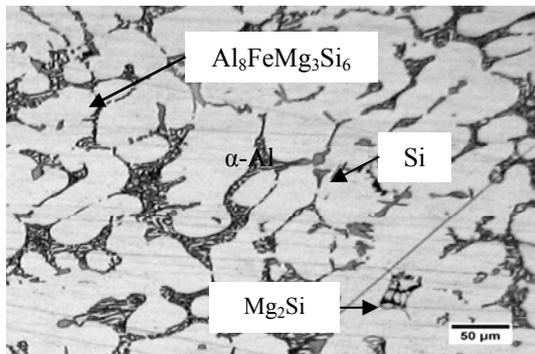
Figure 2: Optical micrographs of superheated as-cast AC-M alloy.
