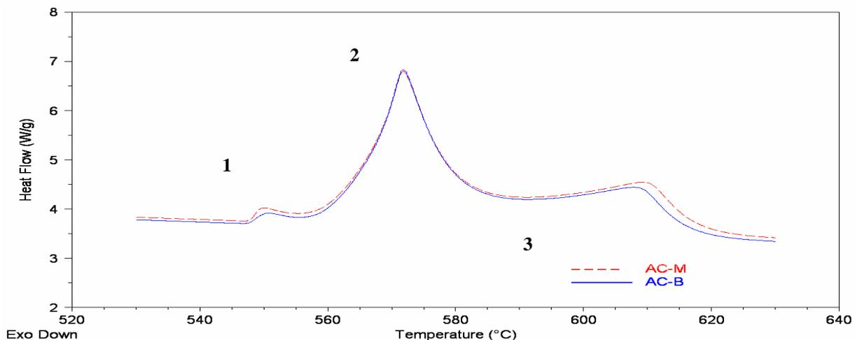
Figure 4: The DSC thermograms of AC-M and AC-B specimens at higher elevated temperatures (530-630°C).
