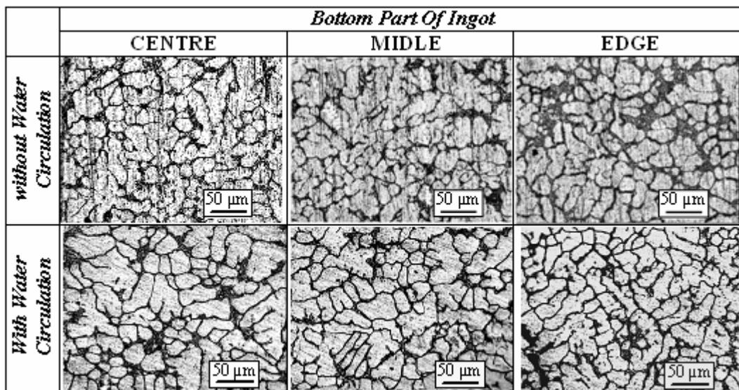
Figure 6: Microstructure of bottom part of CS casting ingot for both with and without water circulation
