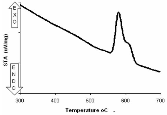
Figure 4: STA curve of the Al-Si alloy recorded during cooling from the molten state
