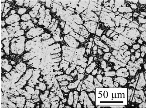
Figure 3: Microstructure of the conventionally cast Al-Si alloy
