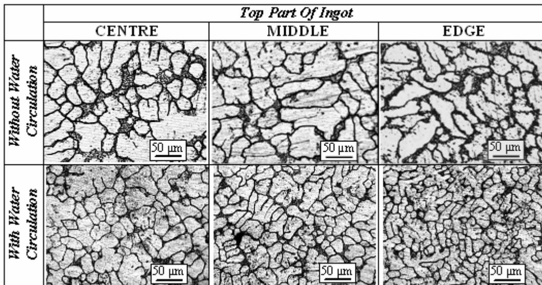
Figure 5: Microstructure of upper part of CS casting ingot for both with and without water circulation
