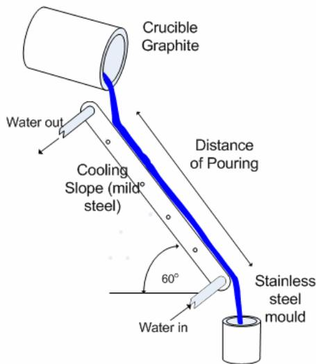
Figure 1: Equipment installation of CS casting used in the present work.
