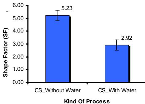
Figure 9: Shape factor of  $\alpha$ -Al particle for CS casting process with and without water
