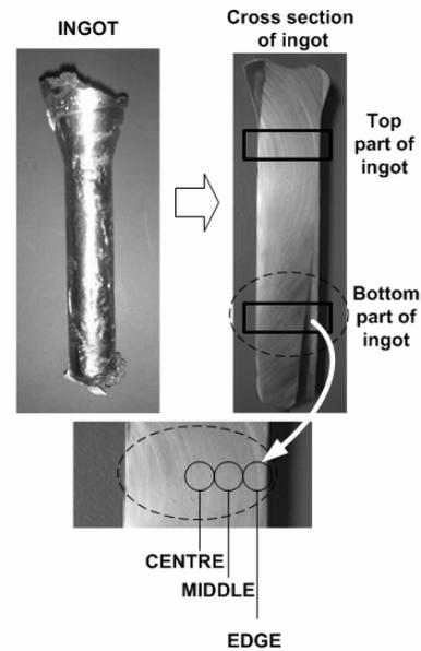
Figure 2: Schematic description of the sample location for metallography
