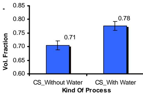
Figure 7: Volume fraction of  $\alpha$ -Al particle for CS casting process with and without water
