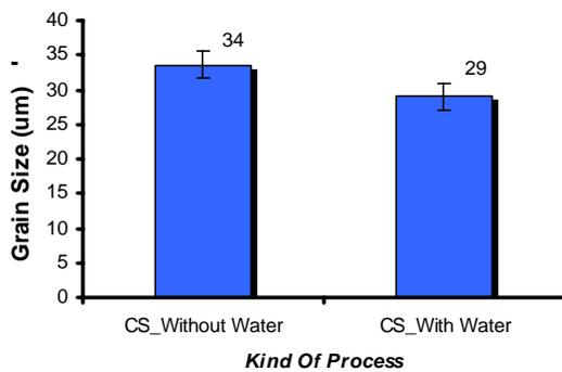
Figure 8: Grain Size of  $\alpha$ -Al particle for CS casting process with and without water
