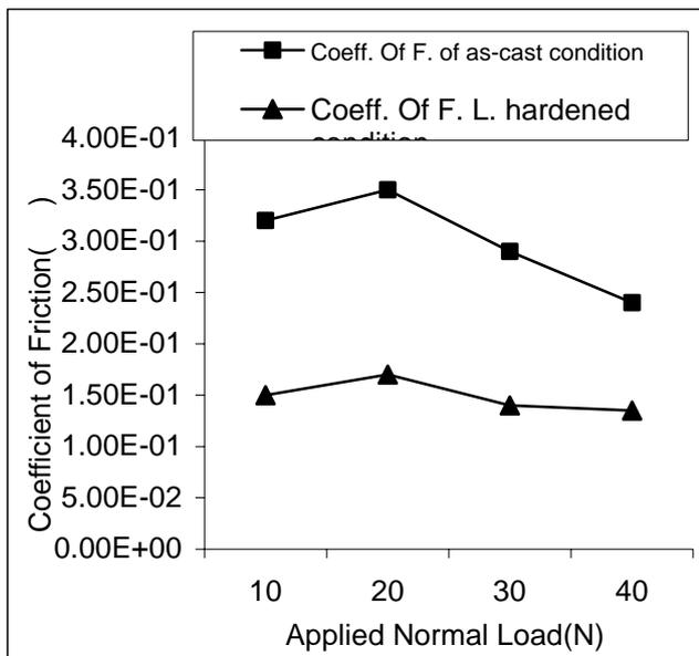
Figure 3: Shows the Effect of Load on The Coefficient of Friction.
