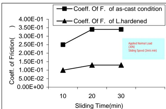
Figure 7: Shows the Effect of Sliding Time on the Coefficient of Friction.
