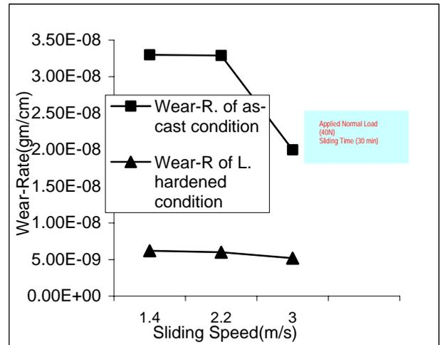
Figure 4: Shows the Effect of Sliding Speed on the Wear Rate.
