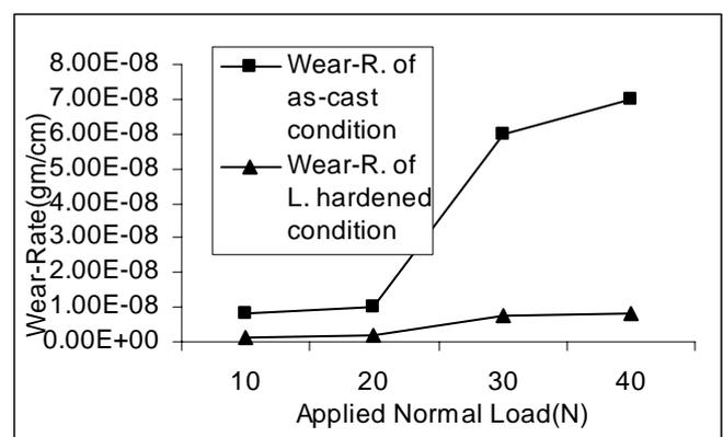
Figure 1: Shows the Effect of Load on The Wear Rate.
