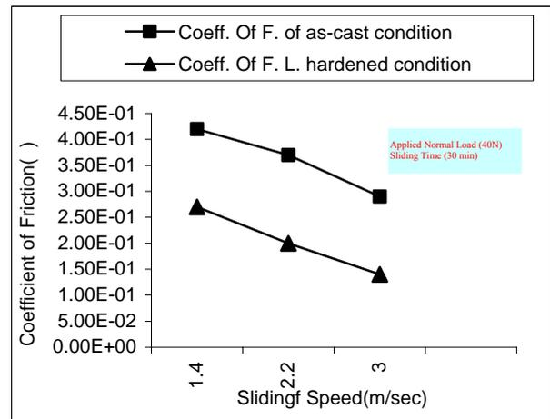
Figure 5: Shows the Effect of Sliding Speed on the Coefficient of Friction.
