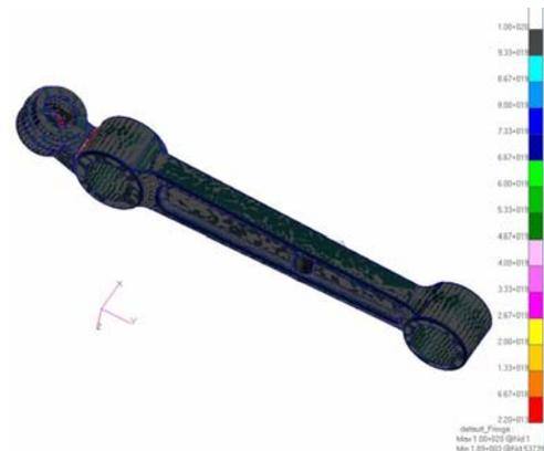
Fig. 6: Model fatigue life contour
