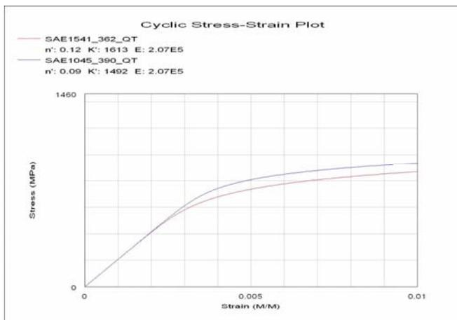
Fig. 7: Cyclic stress-strain curves for SAE1541\_362\_QT and SAE1045\_390\_QT steel
