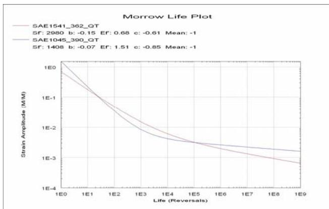
Fig. 9. Morrow life plot for medium carbon steel SAE1541\_362\_QT and SAE1045\_390\_QT
