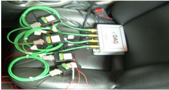
Fig. 3: The setup of fatigue data acquisition system data collection.
