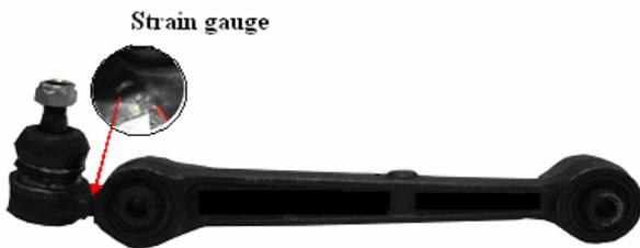
Fig. 4: Strain gauge location on the lower suspension arm
