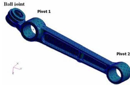
Fig. 2. Finite element model of the lower suspension arm
