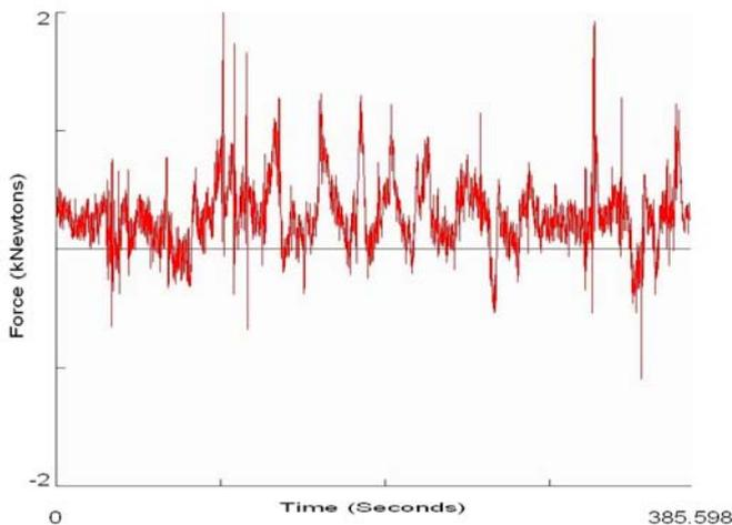
Fig. 5: Experimental loading history for the lower suspension arm.
