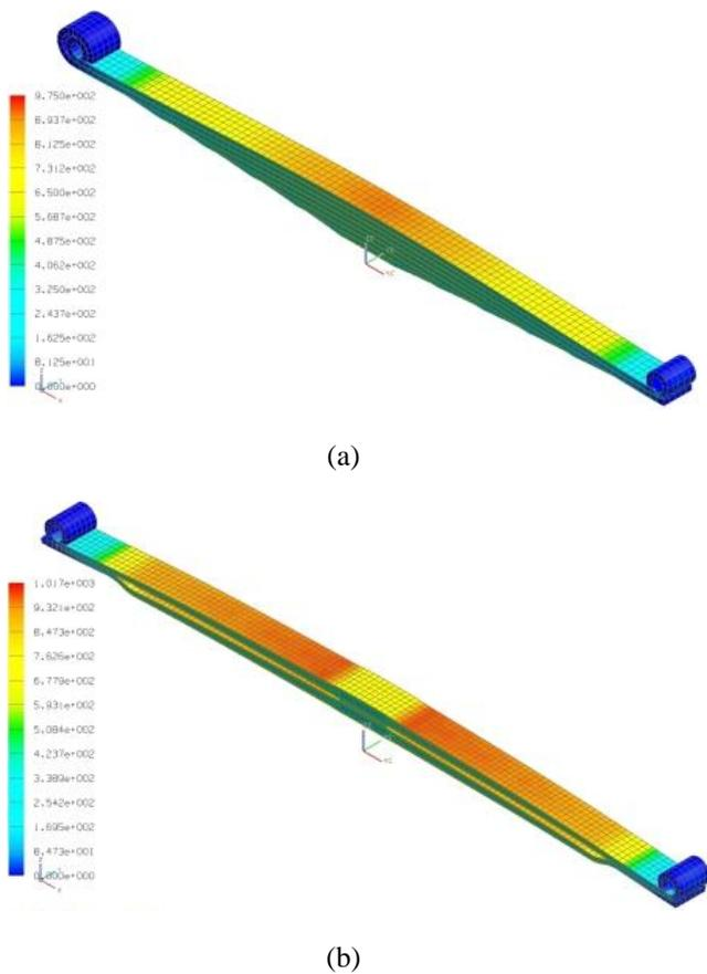
Fig. 4. : Stress distribution areas on a particular component: (a) multi-leaf spring, (b) parabolic spring
