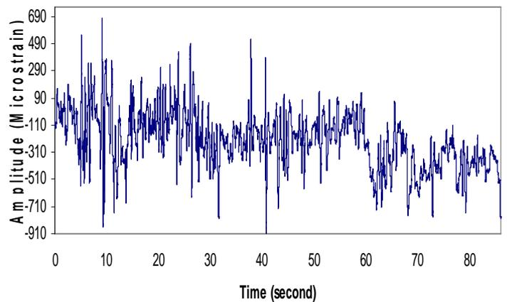
Fig. 3. : Variable amplitude loading signal which was collected from the data collection work
