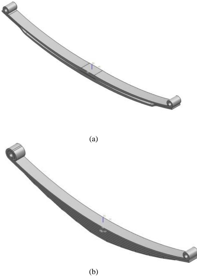
Fig. 1. Geometry schematic of (a) multileaf spring and (b) parabolic spring
