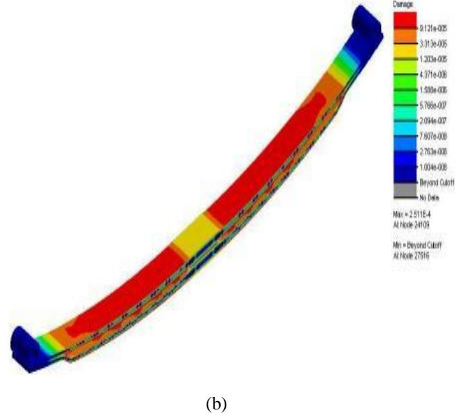
Fig. 7.: Load FEA-based fatigue prediction: (a) Multi-leaf spring, (b) Parabolic spring
