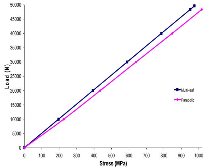
Fig. 5.: Load vs. Stress graph of multi-leaf and parabolic spring
