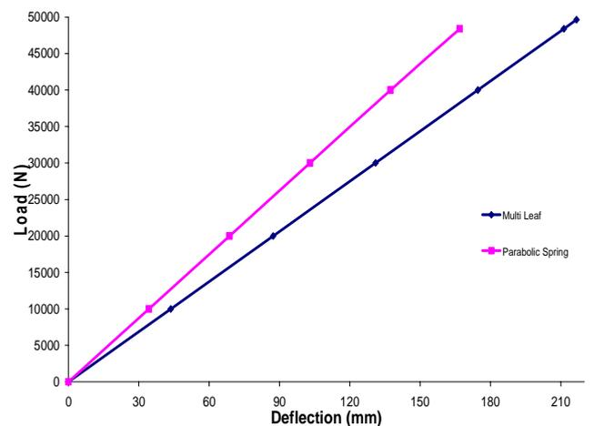
Fig. 6. : Load vs. deflection graph of multi-leaf and parabolic spring
