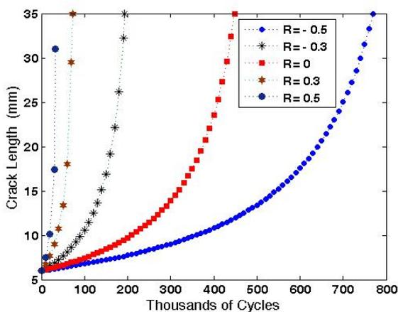
Fig. 7.: Fatigue Crack Growth with Different Stress Ratio
