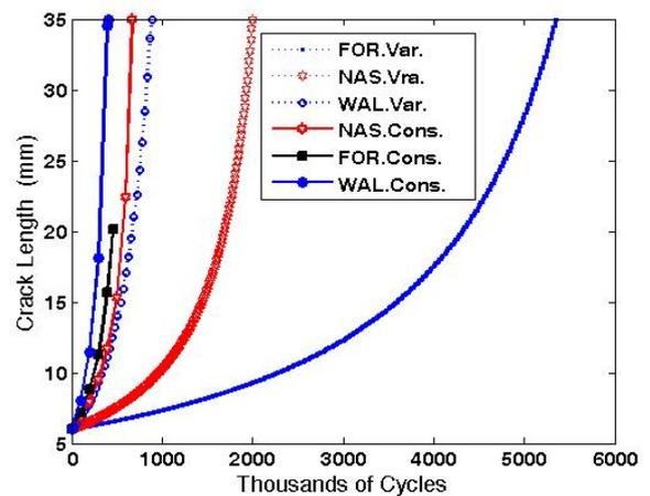
Fig.4.: Fatigue Crack Growth of Thin Wall Tube with CAL and VAL using Different FCG Models
