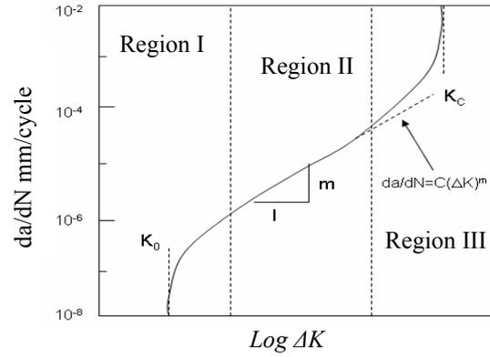
Fig. 1.: Typical  $da/dN$  versus  $\Delta K$  curve
