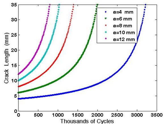
Fig. 5.: Fatigue Crack Growth for Different Initial Crack Length
