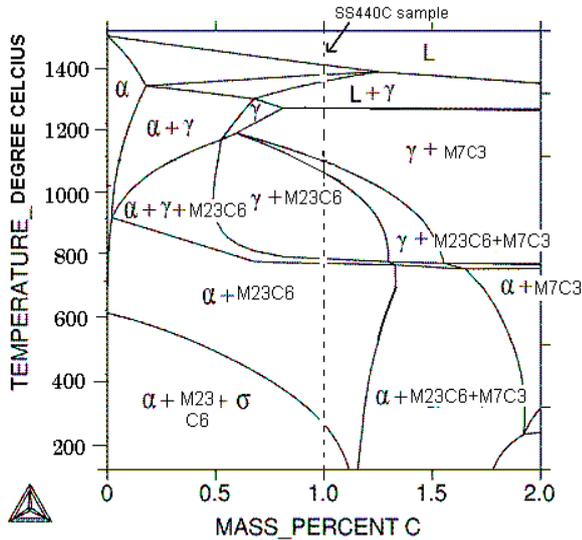
Figure 1. The Equilibrium Phase Diagram of 440C Steel
