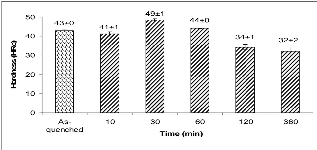
Figure 3. Hardness (HRC) Values of As-quenched and As-tempered Samples
