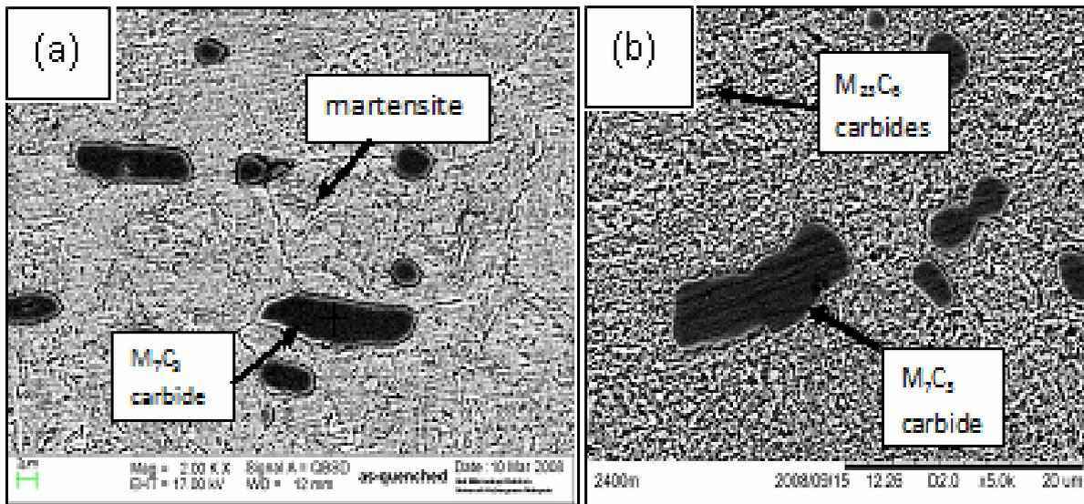
Figure 2. The Scanning Electron Micrograph of (a) As-quenched and (b) As-tempered Sample.
