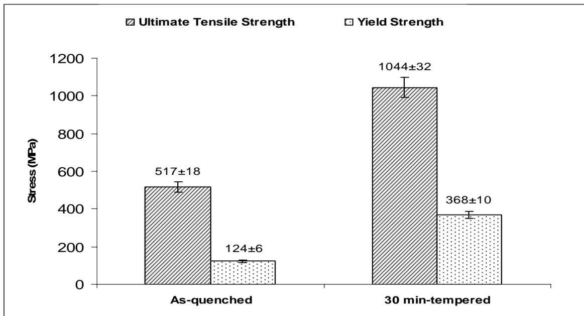
Figure 4. Tensile Properties of Heat-treated Samples.
