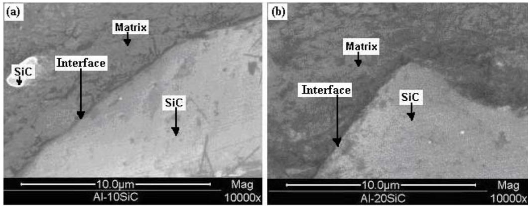
Fig. 4: Micrograph showing good cohesion at the interface between the Al-Si matrix and SiC particles for Al-Si/10% SiC<sub>p</sub> and Al-Si/20% SiC<sub>p</sub> respectively.
