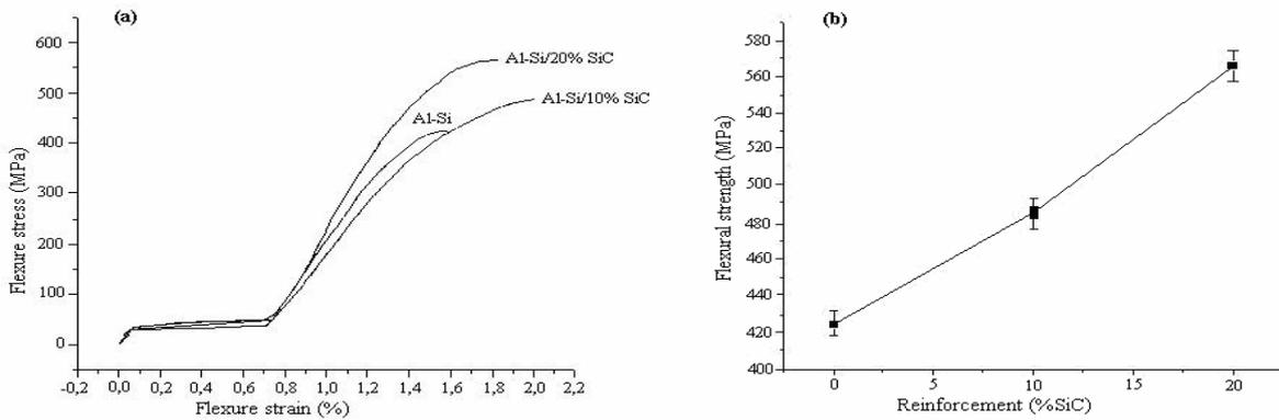
Fig. 1: (a) The flexural behaviour of Al-Si/SiC<sub>p</sub> composites and (b) Flexural strength versus SiC<sub>p</sub> content of the composites.
