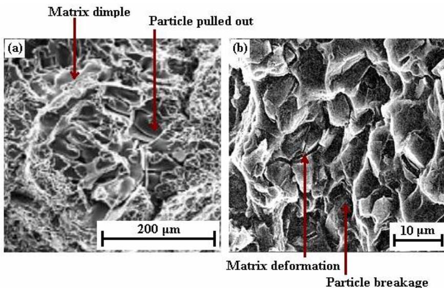
Fig. 6: Micrographs of the fracture surfaces show (a) matrix dimples and pullout of the SiC<sub>p</sub> (b) broken particle and matrix failure or deformation.
