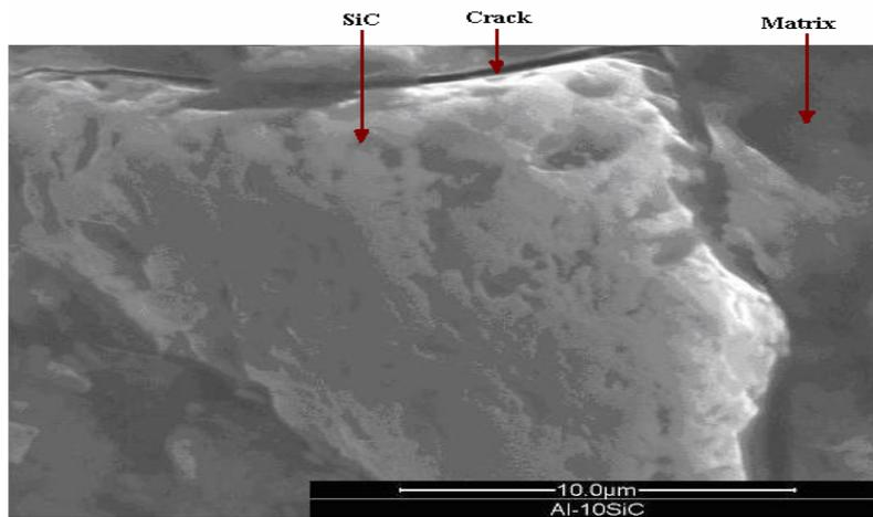
Fig. 5 Crack initiation at SiC<sub>p</sub> due to debonding at the interface
