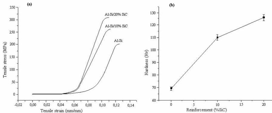
Fig 2: Mechanical properties of composites; (a) Tensile properties of Al-Si/SiC<sub>p</sub> composites (b) Effect of SiC<sub>p</sub> on hardness of Al-Si/SiC<sub>p</sub> composites.
