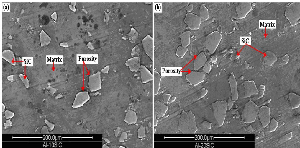
Fig. 3: Fractographs of crack initiation at the fractured SiC particles for Al-Si/10% SiC<sub>p</sub> and Al-Si/20% SiC<sub>p</sub> respectively.
