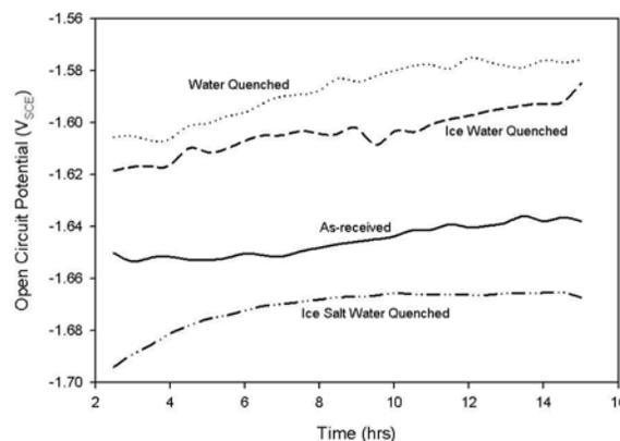
Fig. 2.  $E_{oc}$  Value of Mg Alloy Anode Solution Treated at 150 °C in Different Cooling Method in Iced Salt Water
