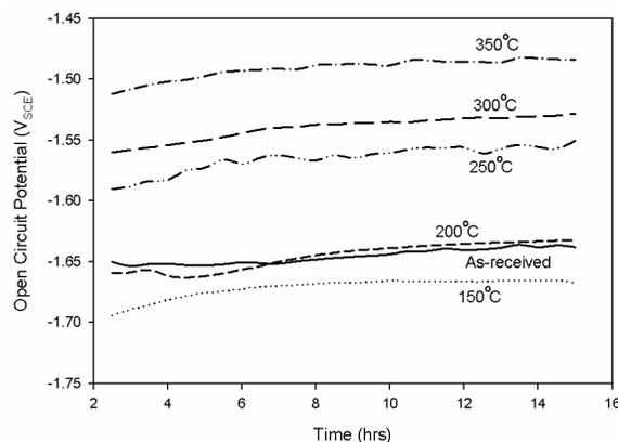
Fig 1:  $E_{oc}$  Value of Mg Alloy Anode Solution Treated at Different Temperature and Cooled in Iced Salt Water.
