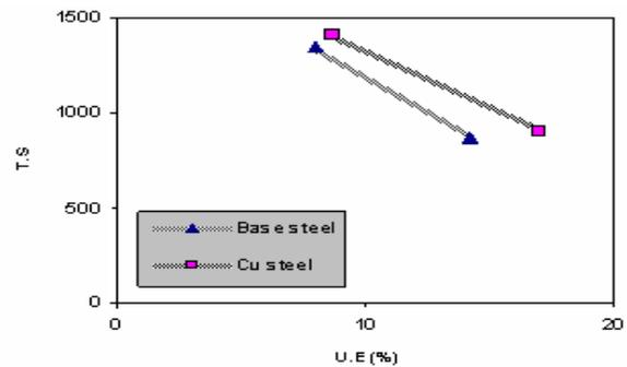
Fig. 5 Relation between U.E (%) and T.S in Cu and Base steel, which are annealed at dual phase steel region and water quenched.
