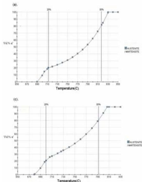
Fig. 1. Relation between temperature and volume fraction of phases of Base steel (a) and Cu steel (b).
