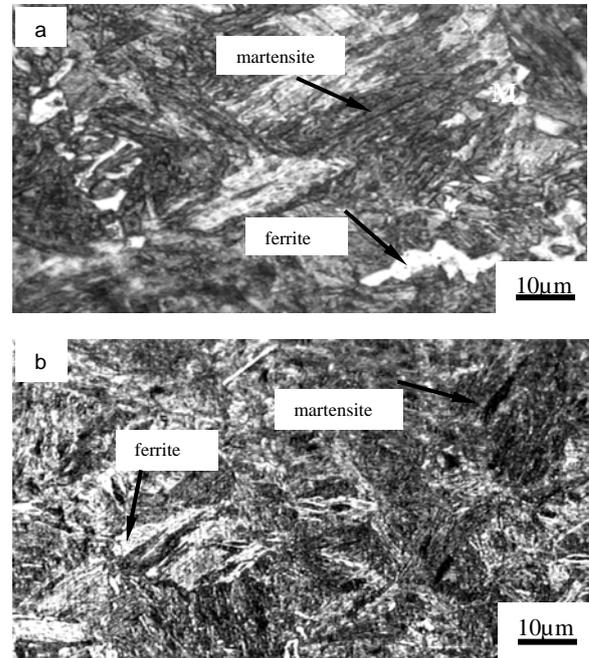
Fig. 3. Microstructures of the annealed steels; Base steel (a) and Cu steel (b). The steels were annealed at temperature to form 80 vol.% of martensite.
