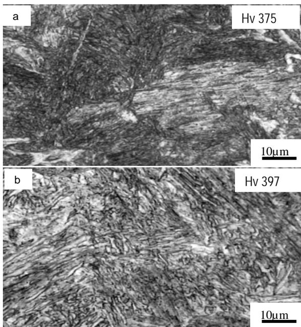
Fig. 2. Microstructures of the as-quenched steels; Base steel (a) and Cu steel (b). The steels were subjected to solution treatment at 1273K for 1.8ks and water-quenching.
