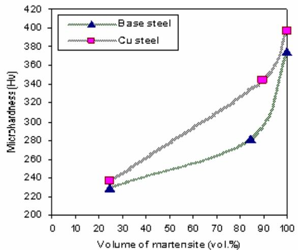
Fig. 4. Relation between Vol.% of martensite and hardness of the steels.
