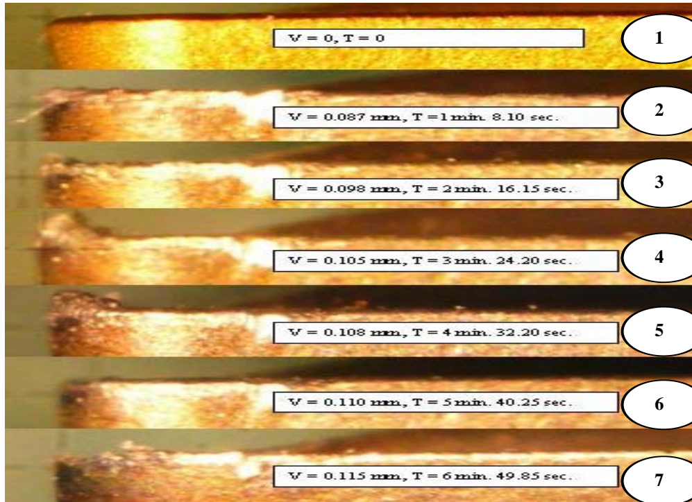
Figure 5. The flank wear progression steps at the initial machining when cutting speed of 55 m/min, feed rate of 0.15 mm/rev and depth of cut of 0.15 mm.
