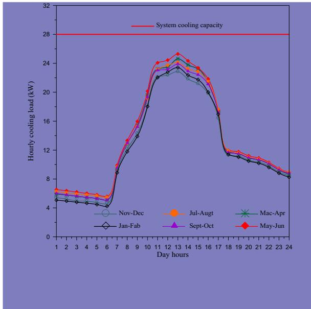
Figure 1: Hourly cooling load distribution at different typical day times around year
