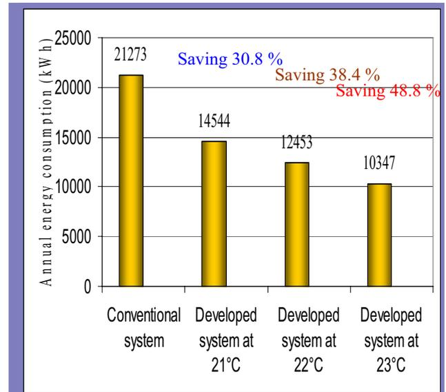
Figure 10: Comparison of yearly energy consumption between the conventional and the developed system for the three temperature settings
