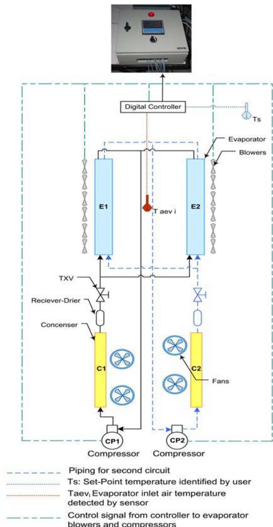
Figure 3: Schematic diagram of the developed multiple-circuit bus air-conditioning
