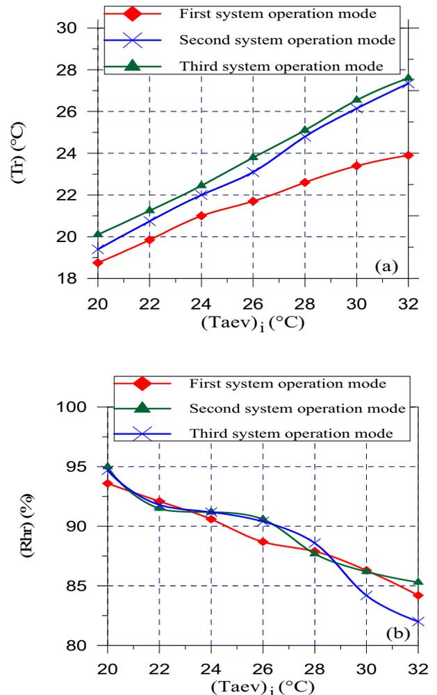
Figure 7: Effect of evaporator inlet air temperature on: (a) space air temperature, and (b) space air relative humidity at the three different modes of the newly developed AC system
