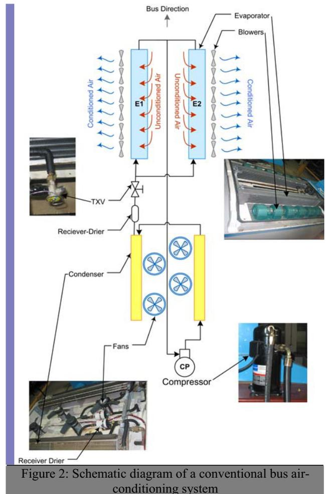
Figure 2: Schematic diagram of a conventional bus air-conditioning system
