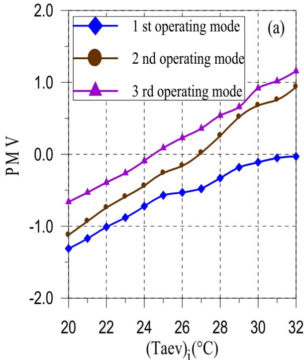
Figure 8: Evaporator inlet air temperature effect on passenger thermal comfort in terms of (a) PMV (b) PPD
