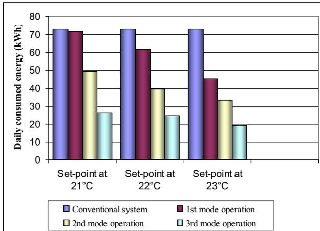
Figure 6: Daily energy consumption for both systems at different set-point temperatures
