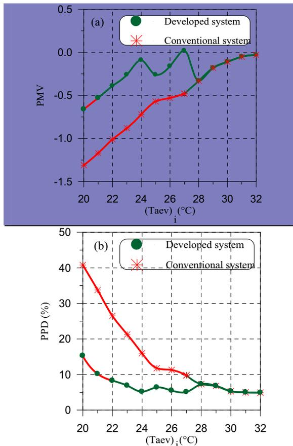
Figure12: Effect of the evaporator inlet air temperature on (a) PMV (b) PPD of the developed and conventional systems
