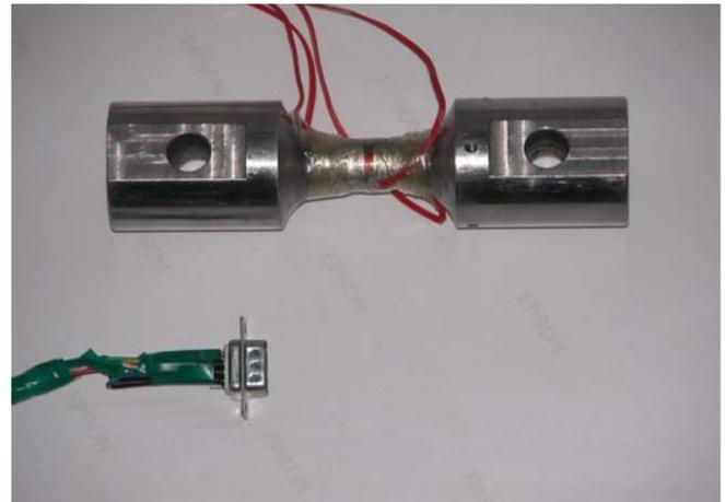
Figure 6: Developed motion resistance transducer.
