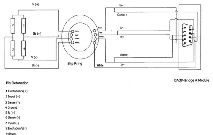
Figure 4: Torque transducer electrical wiring system
