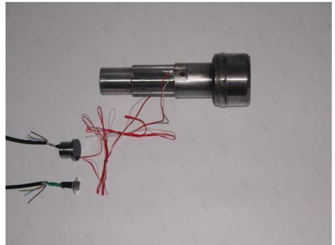
Figure 3: Developed torque transducer
