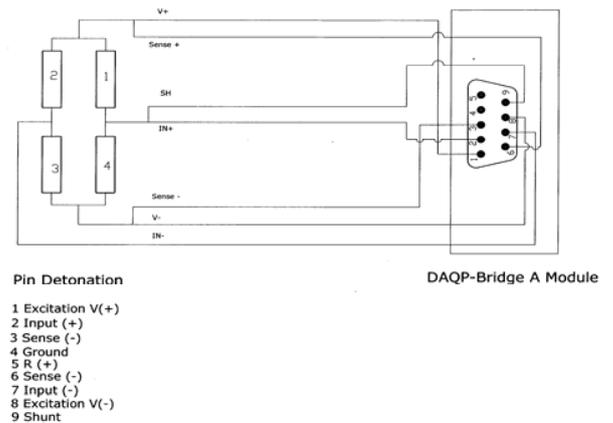
Figure 7: Electrical Circuit Layout
