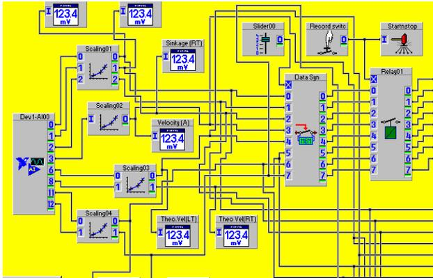
Figure 2. Programming by DasyLab<sup>®</sup> into the DEWETRON-2010.
