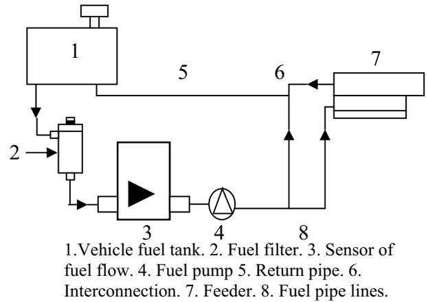
Figure 3 Schematic diagram of the connections of the measuring device with fuel system.
