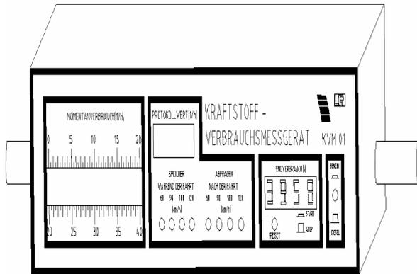
Figure 1 The fuel consumption measuring device installed on each car.
