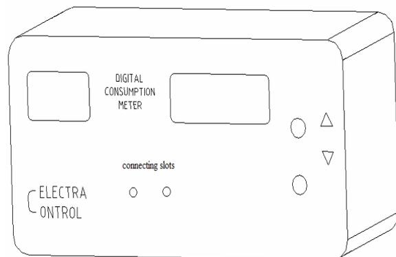
Figure 2 The controller box of the fuel consumption measuring device and its connecting slots.
