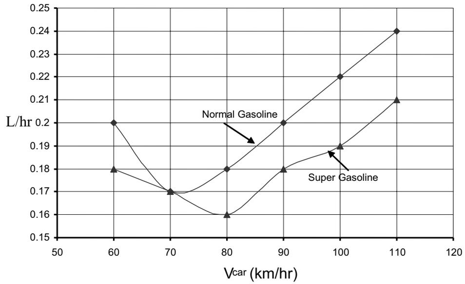
**Figure 8** The effect of fuel type on the rate of fuel consumption.
