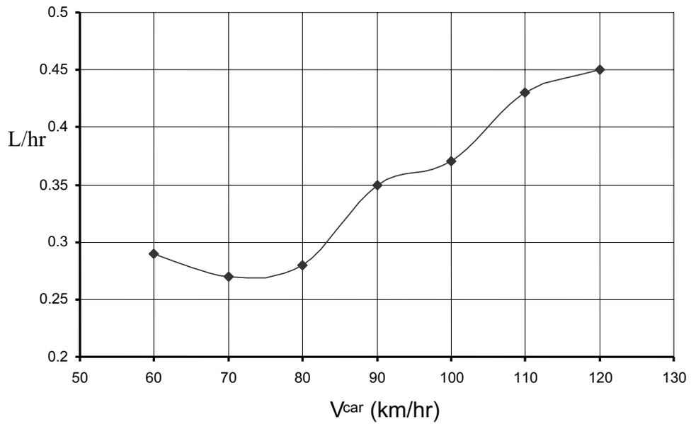
**Figure 7** The effect of vehicle speed on the rate of fuel consumption.
