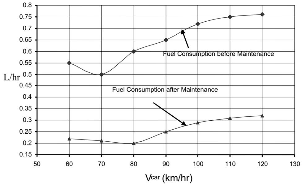
**Figure 10** The effect of vehicle maintenance on the rate of fuel consumption.
