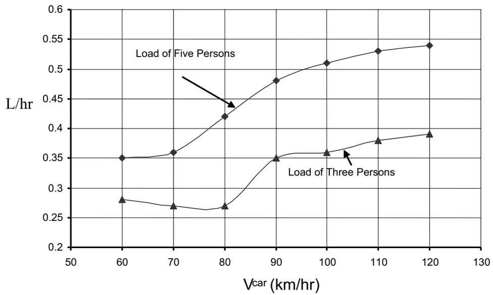
**Figure 9** The effect of load on the rate of fuel consumption.
