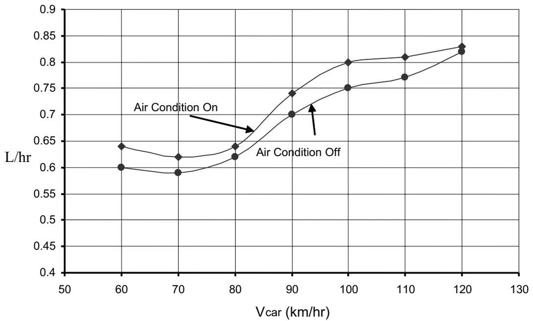
**Figure 5** The effect of air-conditioning operation on the rate of fuel consumption.
