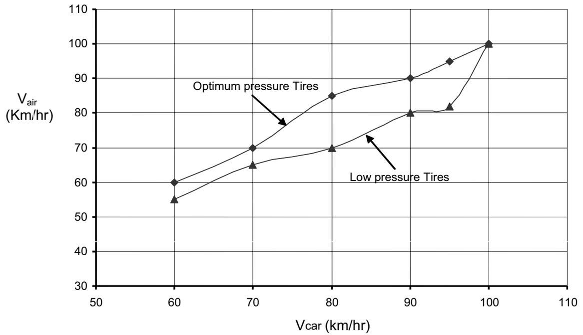
**Figure 4** The effect of tires condition on the air flow on car.
