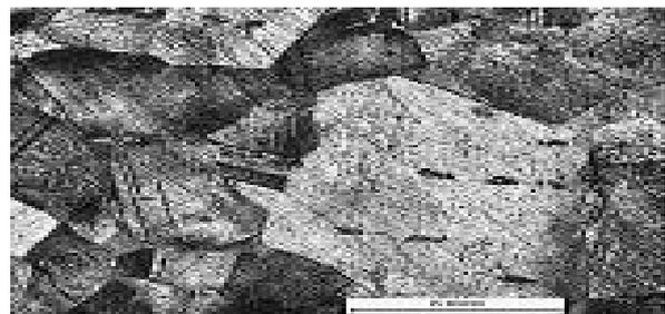
Figure 1: Austenite grains of Hadfield's steel with twins
