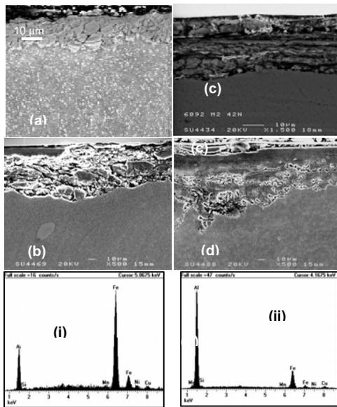
Fig. 2.: Higher magnifications of longitudinal cross-sections of A2124 at (a) 23N (b) 140N and A6092 at (c) 42N and (d) 140N. A corresponding EDS analysis of A6092 cross section at 140N against M2 are shown
