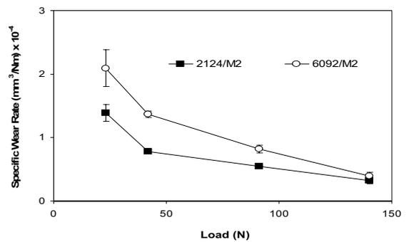
Fig. 3.: Specific wear rate of both alloys as a function of load.
