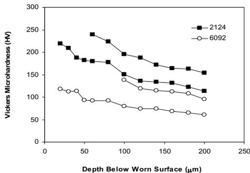
Fig. 4.: Hardness profile of alloys as a function of the deformed depth at 23N and 140N. The first datum corresponds to the depth where the first metal is found below the MML.
