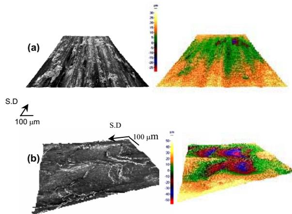
Fig. 1.: Digital Elevation Models of (a) A2124 and (b) A6092 alloy worn surface against M2 at 140N showing the texture image. S.D represents the sliding direction.
