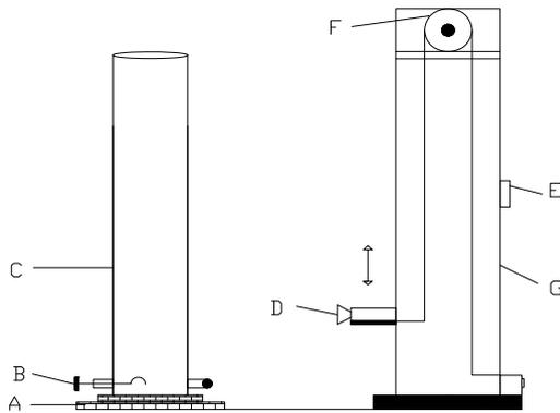
A = Sturdy Base; B = Rotating Spoon; C = Cylindrical test rig (0.125 m or 0.40 m diameter), D = Video camera; E = Variable speed motor; F = Pulley; and G = Camera lifting device.
