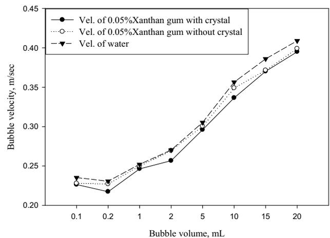
Figure 2 Comparison of bubble rise velocity for water, 0.05% xanthan gum and crystal suspension at 1 m height.
