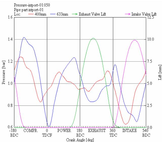
Fig. 9. Intake Port Pressure for 400 mm and 633 mm at 6000 rpm
