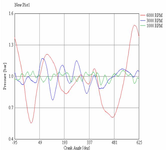
Fig. 7. Intake port pressure vs. crank angle
