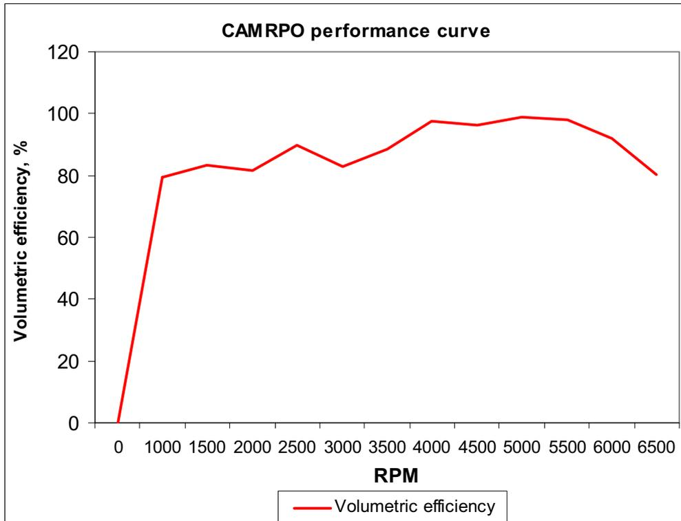
Fig. 8. CAMRPO volumetric efficiency curve
