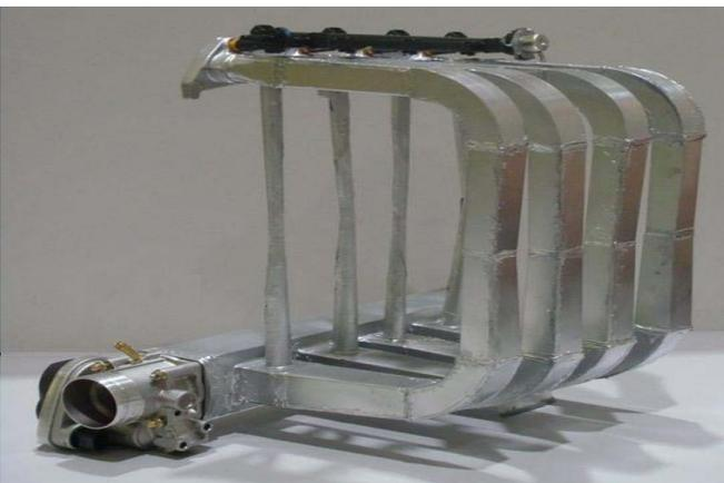
Fig. 16. Fabricated NDIM
