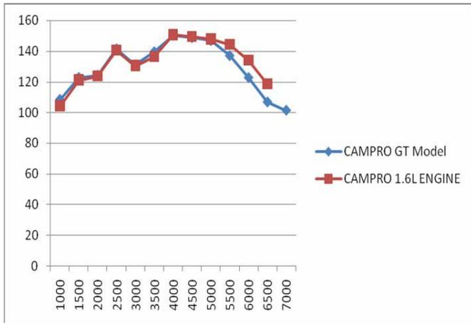
Fig. 2. Torque vs RPM for the CAMPRO 1.6L Engine and its GT Model
