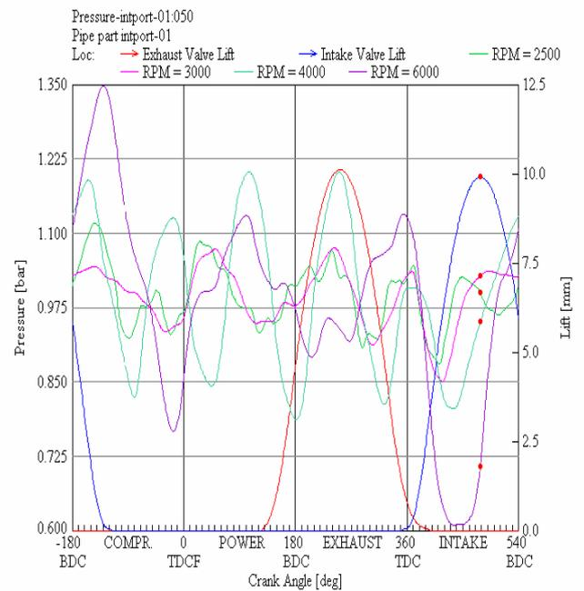
Fig. 5. Intake Port Pressure and Intake Valve Lift vs. Crank Angle
