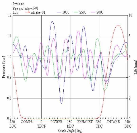
Fig. 10. Intake Port Pressure at 2000, 2500 and 3000 rpm
