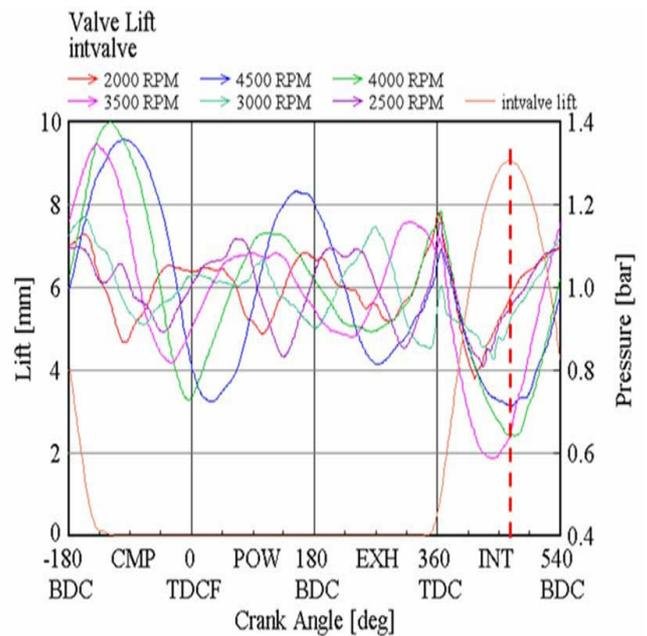
Fig. 15. The pressure wave of 2000 RPM – 4500 RPM
