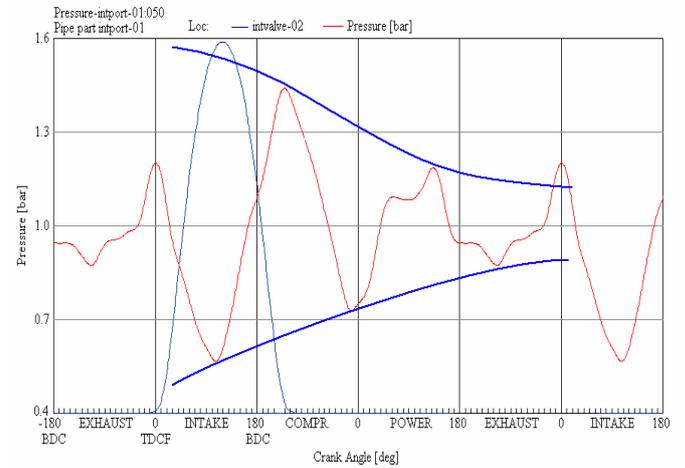
Fig. 4. Valve Timing and Pressure Oscillation in Intake Manifold
