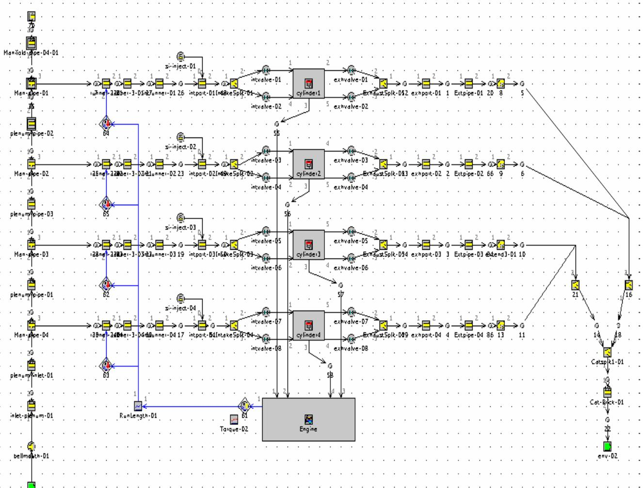
Fig. 18. Continuously Variable Intake Manifold GT Model
