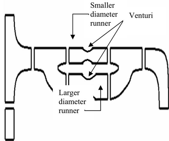
Fig. 11. Intake Runner of NDIM Model
