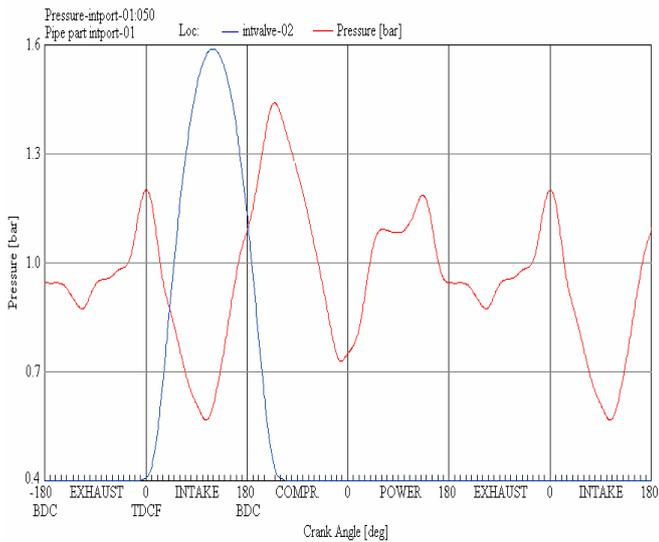
Fig. 3. Intake Port Pressure vs. Crank Angle at 6000 rpm
