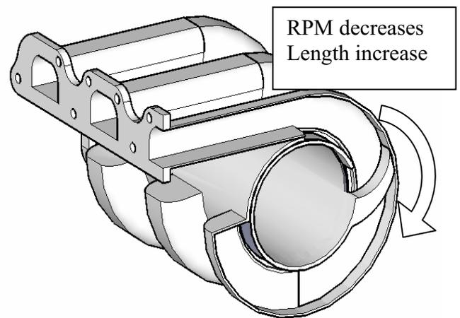
Fig. 17. Continuously Variable Intake Manifold Model
