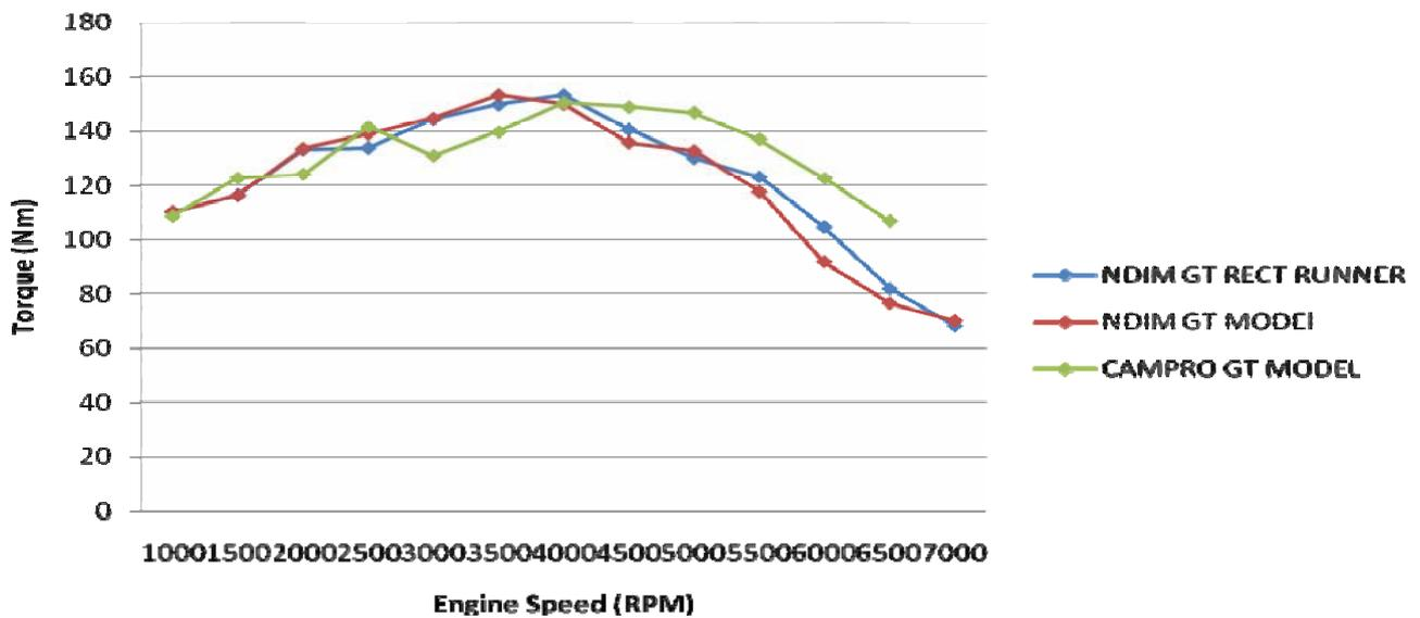
Fig. 14. Performance Test Result Comparison between CAMPRO, CAMPRO GT and NDIM GT Model - Torque
