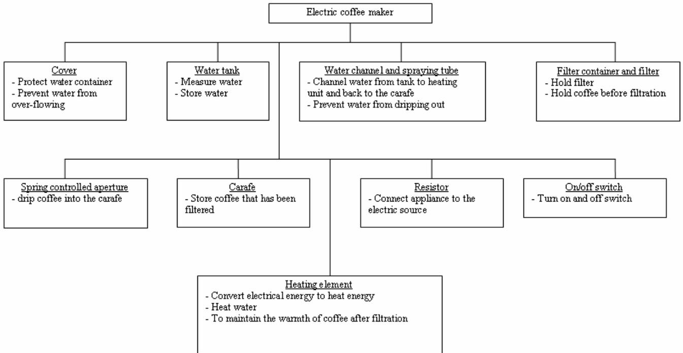
Figure 2 Physical and functional decomposition chart for the electric coffee maker
