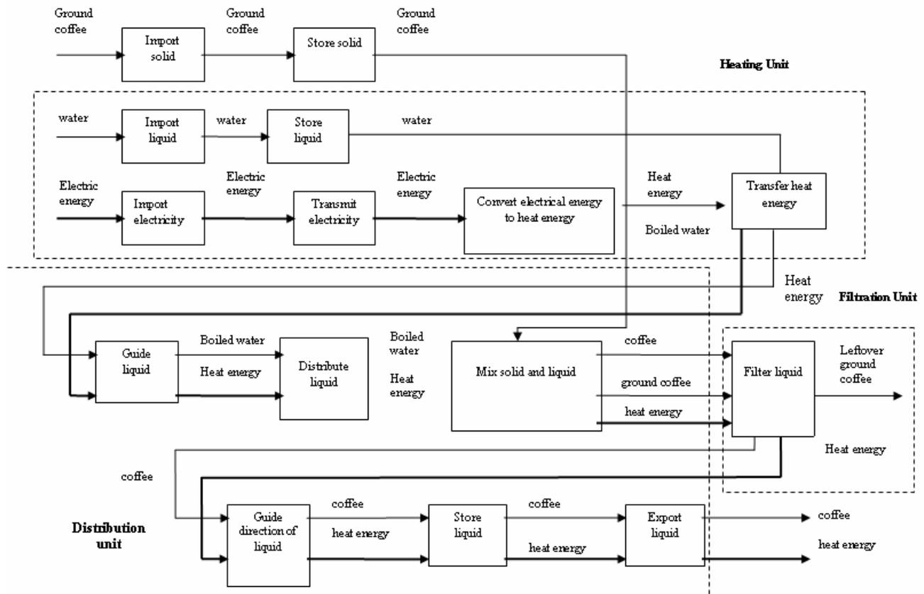
Figure 3 Functional model of the electric coffee maker
