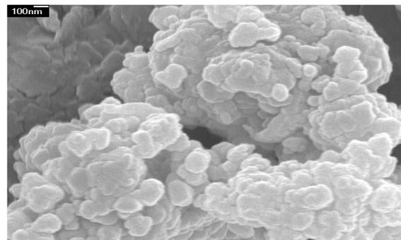
Figure 5: SEM photograph of hydroxyapatite powder.
