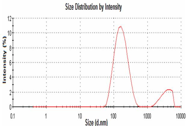
Figure 6: Distribution particles of hydroxyapatite powder as measured using nanoparticle sizer.
