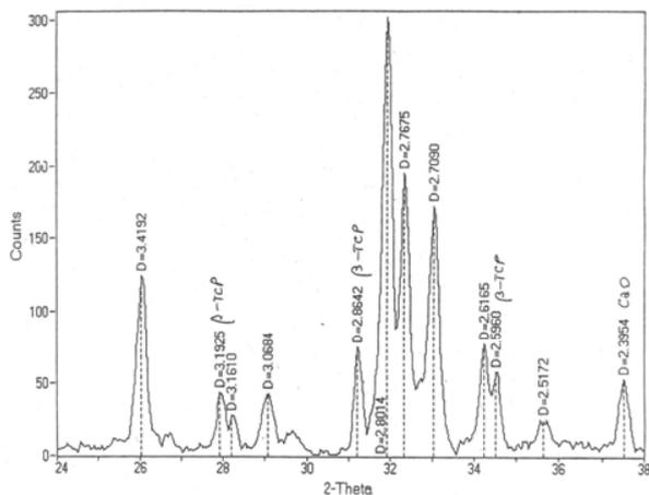
Figure 3: XRD pattern of hydroxyapatite powder mixed with TCP and CaO obtained before the purification process.
