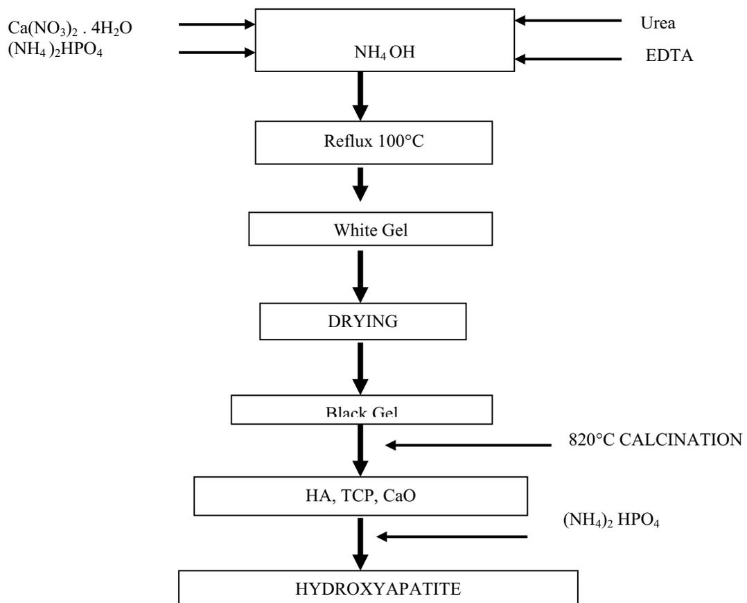
Figure 1: Scheme of Hydroxyapatite preparation via Sol-Gel Method.
