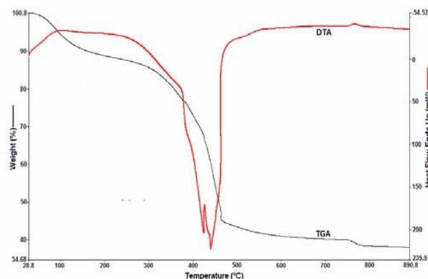
Figure 2: DTA-TG curve of the gel dried at 340°C.
