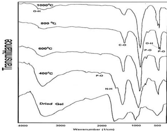
Figure 7: FTIR spectra of dried black gel and the sol-gel hydroxyapatite powder obtained after calcinations at temperatures of 400, 600, 800, and 1000°C.
