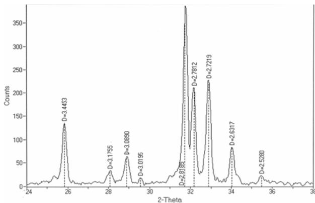
Figure 4: XRD pattern of pure hydroxyapatite powder obtained after the purification process.
