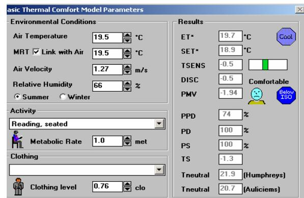
Figure 3 Thermal comfort results computed using ASHRAE Thermal Comfort Software
