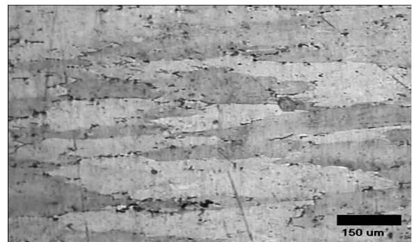
Fig 2(a) Microstructure of the as-received aluminum alloy (sample A-0)
