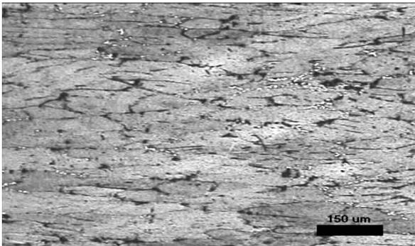
Fig 2(b) Microstructure of aluminum alloy heated to 550 °C then slowly cooled (sample B)
