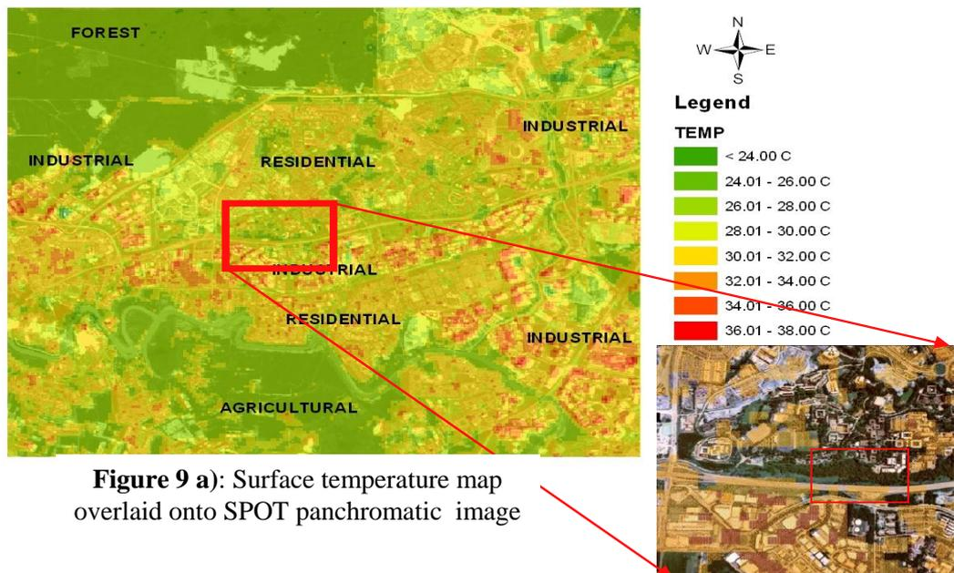
**Figure 9 a):** Surface temperature map overlaid onto SPOT panchromatic image
