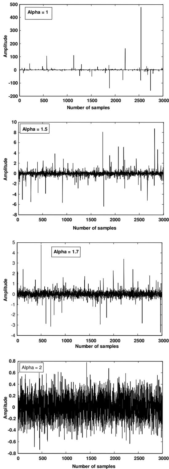
Fig. 3. Symmetric Alpha-Stable Noise with  $\alpha = 1, 1.5, 1.7$  and  $2$ .
