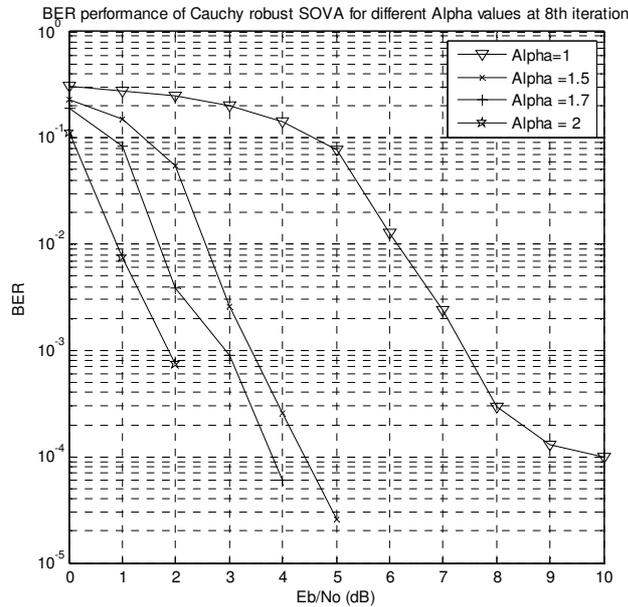
**Fig. 10. BER Performance for Robust SOVA with Bayesian Cauchy Metric over S $\alpha$ S Channel with Different Alpha Values at 8<sup>th</sup> iteration.**
