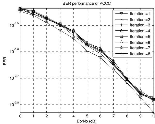
**Fig. 8 BER performance for Conventional SOVA with Bayesian Gaussian Metric over S $\alpha$ S Channel with  $\alpha = 1$ .**
