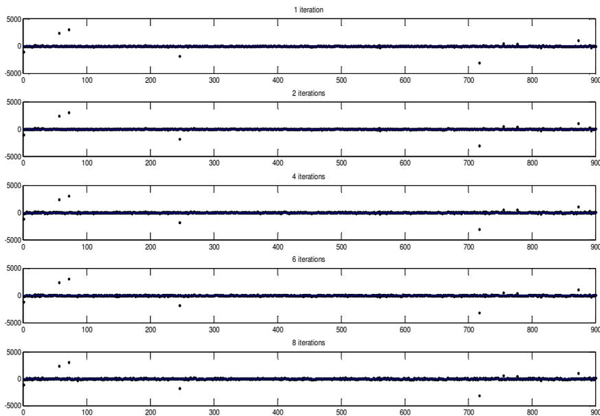
**Fig. 5 Decoded soft LLR Output of Gaussian-based SOVA over SαS Channel with  $\alpha = 1$  at  $E_b/N_o = 8$  dB.**
