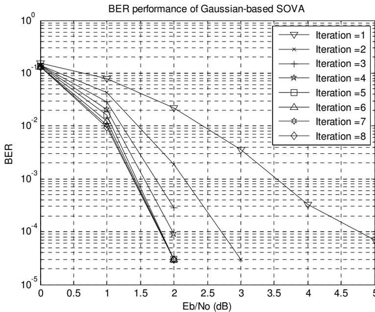
**Fig. 7. BER Performance for Conventional SOVA with Bayesian Gaussian metric over AWGN Channel.**
