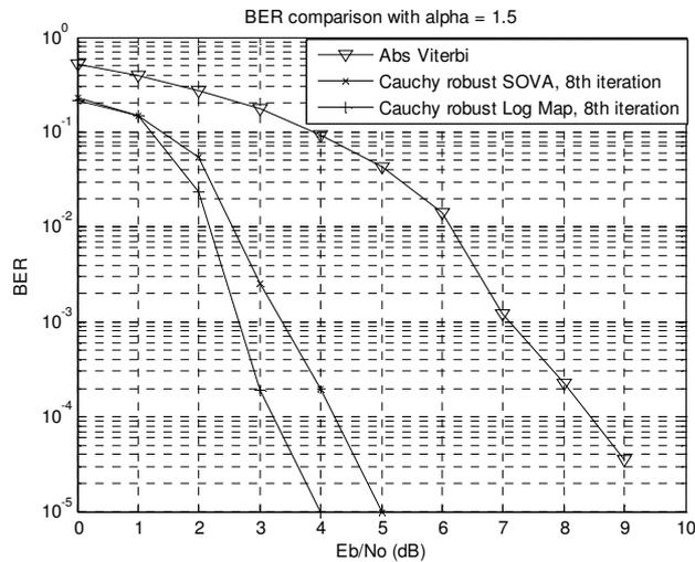
**Fig. 11. BER Performance Comparison of Absolute Viterbi, Bayesian-Cauchy Robust Log Map and Bayesian-Cauchy Robust SOVA over S $\alpha$ S Channel with Alpha = 1.5 at 8<sup>th</sup> iteration.**
