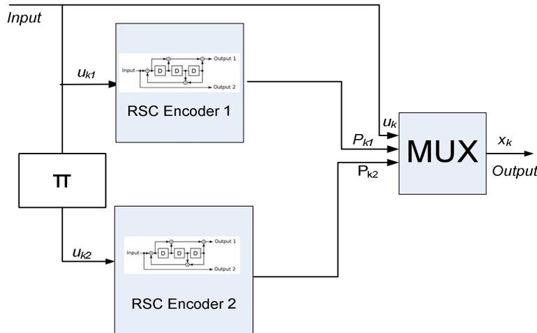
Fig. 1. PCCC Encoder with Code Rate  $r = 1/3$ .
