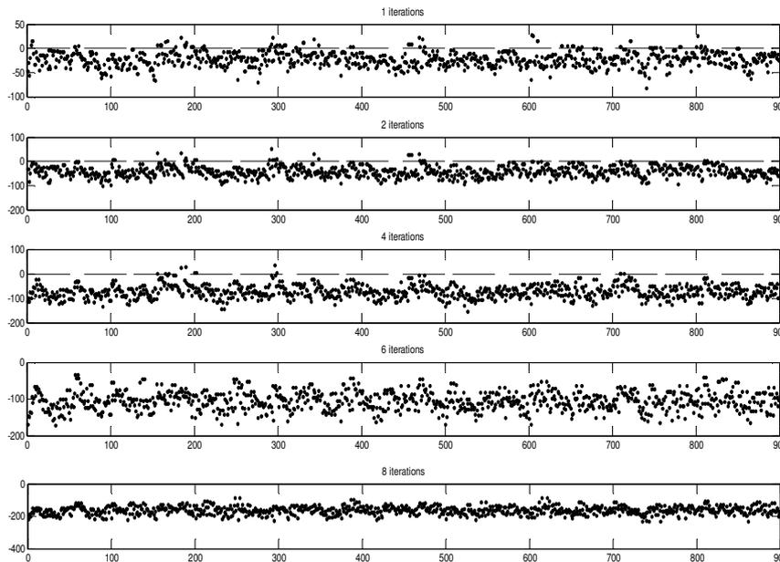
**Fig. 4. Decoded soft LLR Output of Gaussian-Based SOVA over AWGN Channel at  $E_b/N_o = 1$  dB.**
