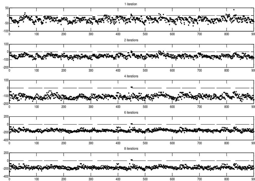
**Fig. 6. Decoded Soft LLR Output of Cauchy-Based SOVA over SαS Channel with  $\alpha = 1$  at  $E_b/N_o = 8$  dB.**
