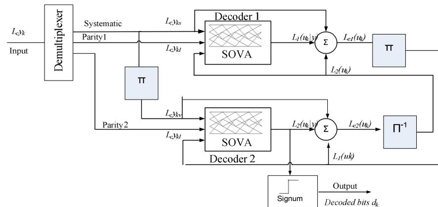
Fig. 2. SOVA Decoder for PCCC.
