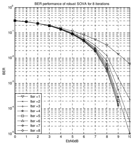
**Fig. 9. BER Performance for Robust SOVA with Bayesian Cauchy Metric over S $\alpha$ S Channel with  $\alpha = 1$ .**
