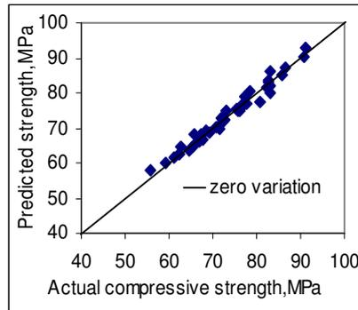
**Fig. 2. Correlation of Experimental Strength with Predicted Strength,  $f_{cf}$ .**
