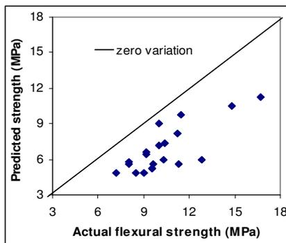
**Fig. 7. Comparison of Predictions with the Experimental Results,  $f_{rf}$  of Earlier Researchers**
