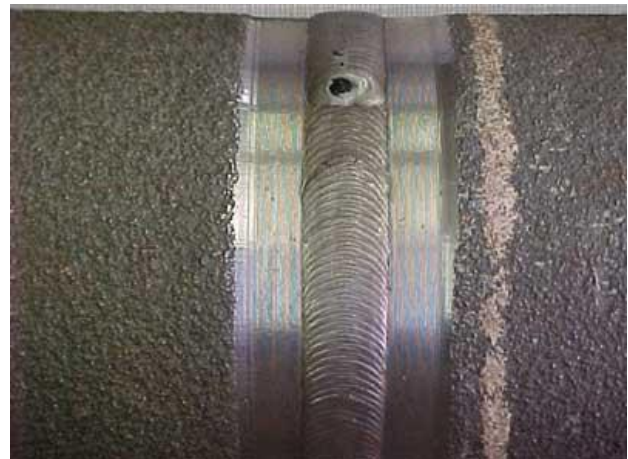
Figure 2 Burn-through as a result of too high amperage (Craig, 2001).
