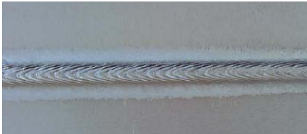
Figure 9 Fillet weld on a 1 mm thick AlMg 3 sheet, CMT welded at a welding speed of 20 mm/min (Fronius Int, 2004).
