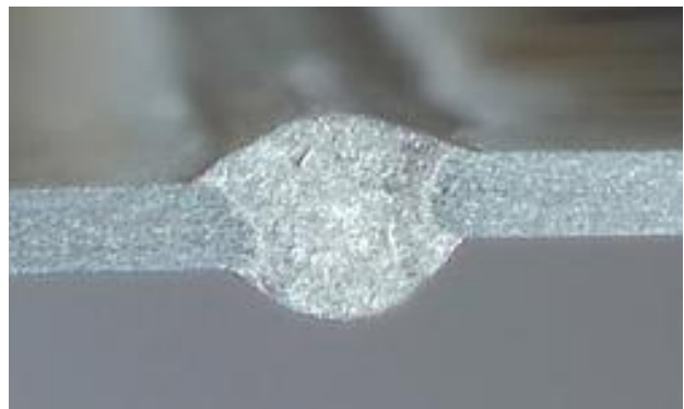
Figure 10 Butt-weld, without weld-pool backing support, on 0.8 mm AlMg 3 sheet with GTAW process (Jiang et al., 2008).
