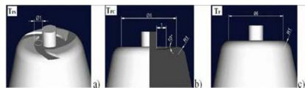
Figure 14 Tools used and their main dimensions fillet + scroll tool (a), fillet + cavity tool (b) and flat fillet tool (c) (De-Giorggi et al., 2009).
